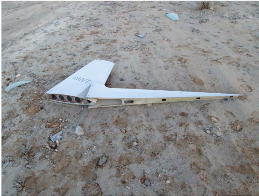
Photo 10 Fin and Vertical Stabilizer
