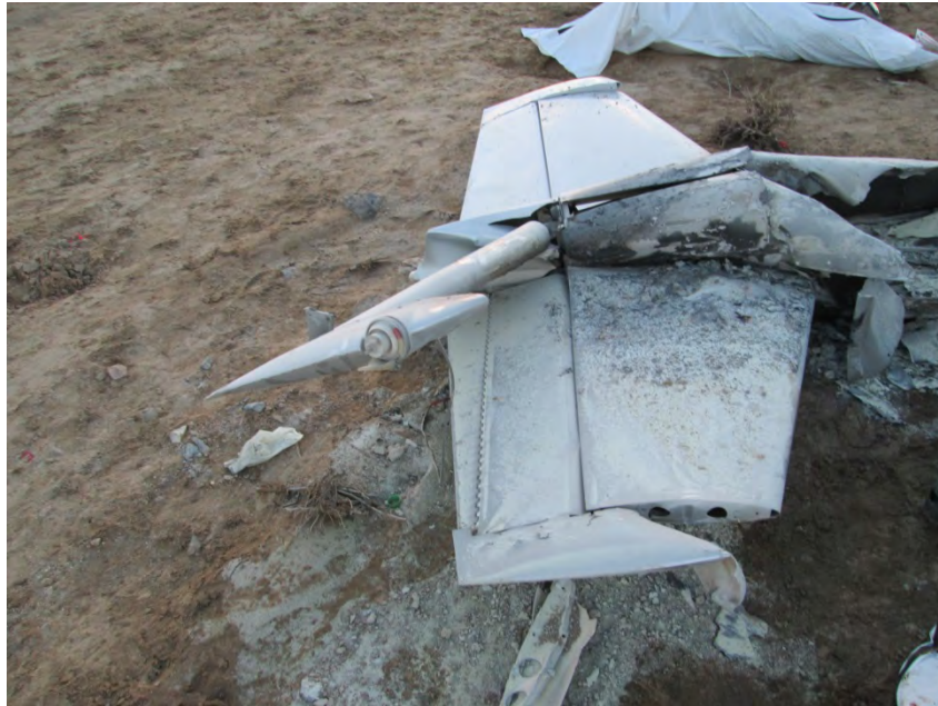
Photo 8 Right Horizontal Stabilizer, Elevator, and Elevator Trim
