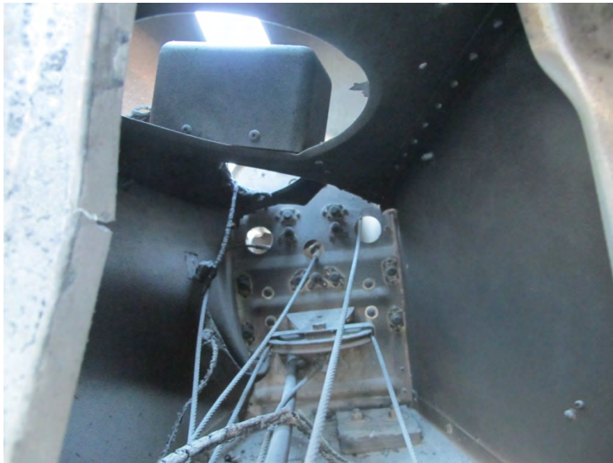
Photo 11 Control Cables in Empennage
