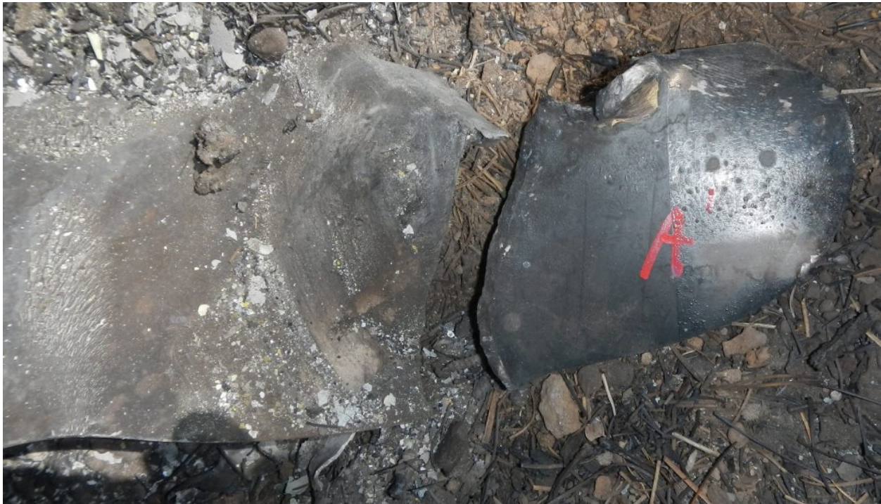
Figure 53 - Blade 'A' with Tip Fragment
