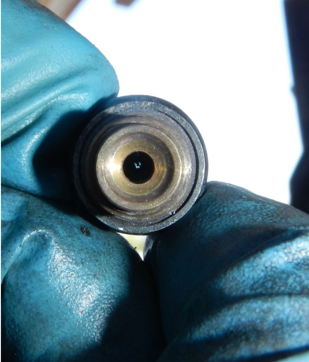
Figure 44 - Injector Nozzle from No. 5 Cylinder (note partial obstruction)
