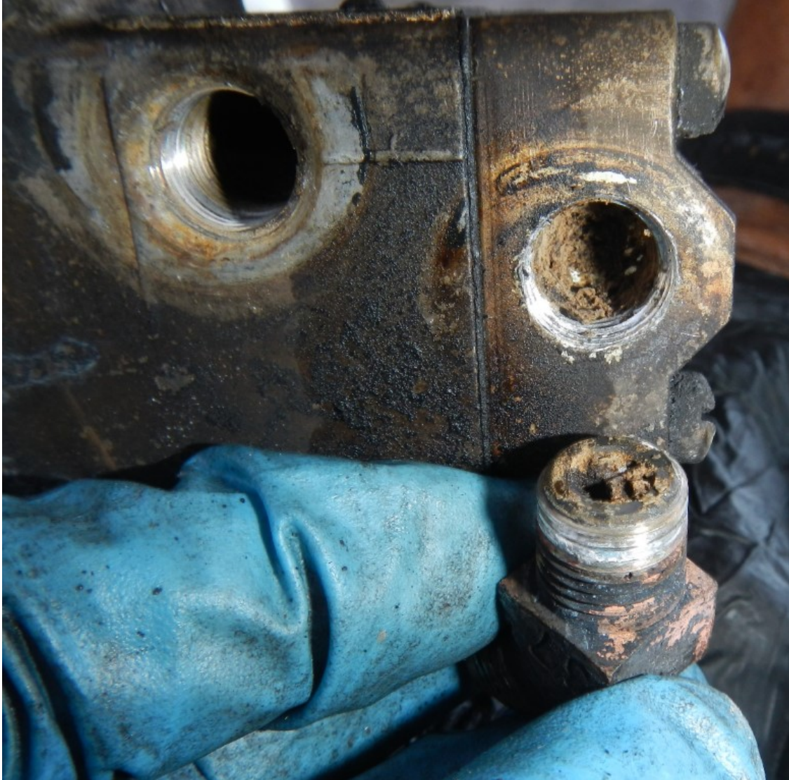
Figure 35 - Debris in EDP
