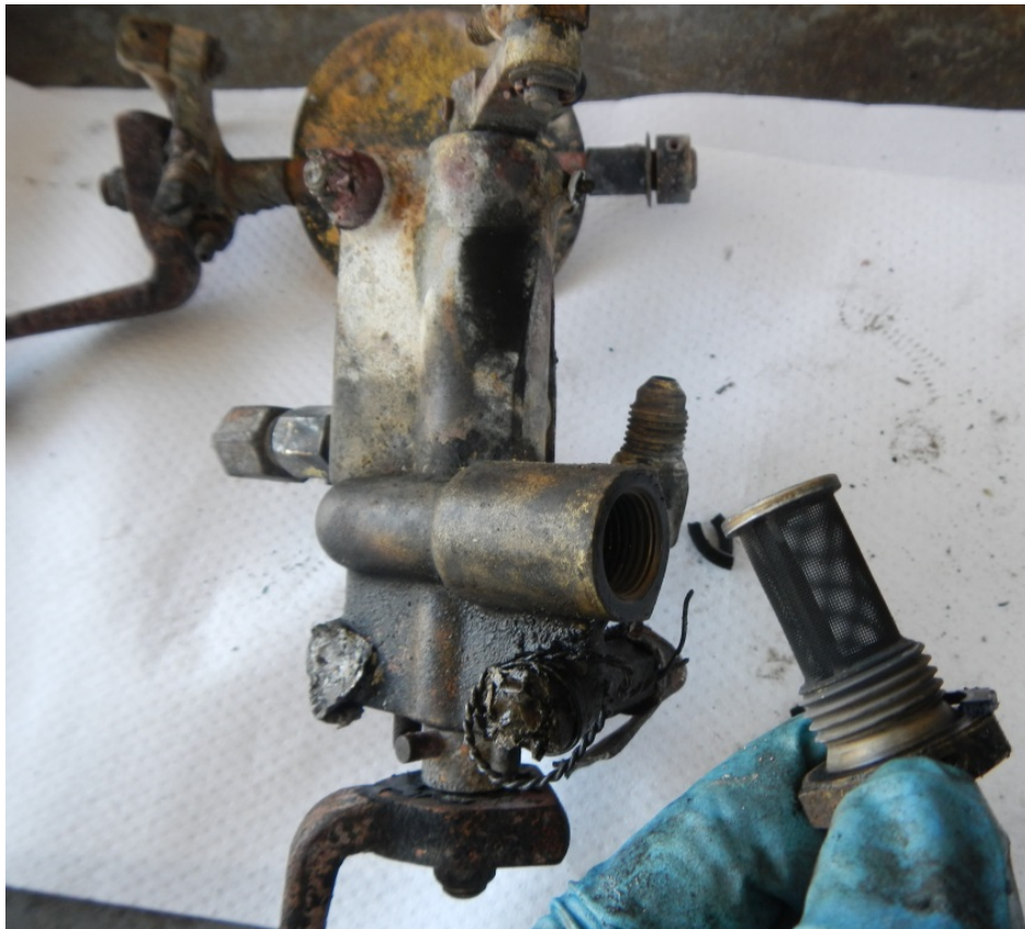
Figure 38 - Metering Unit and Screen
