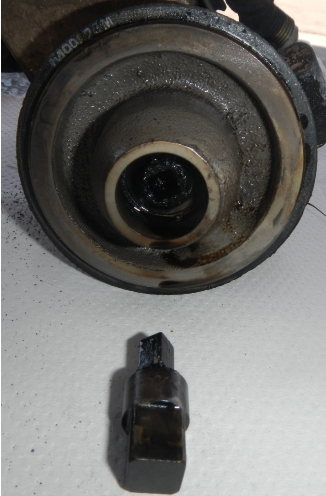
Figure 34 - EDP Drive Link (Intact)
