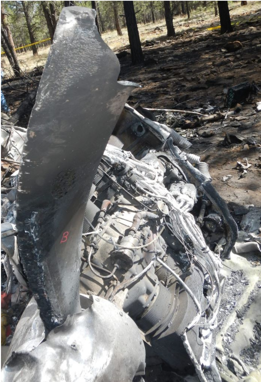
Figure 54 - Blade 'B' with Missing Tip
