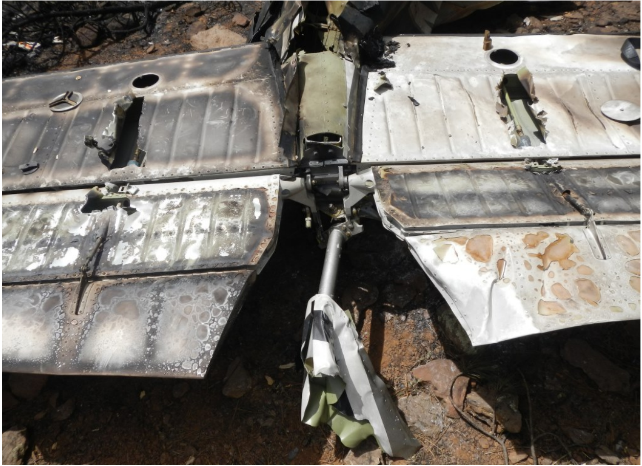
Figure 13 - Stabilizers, Elevators and Rudder Post
