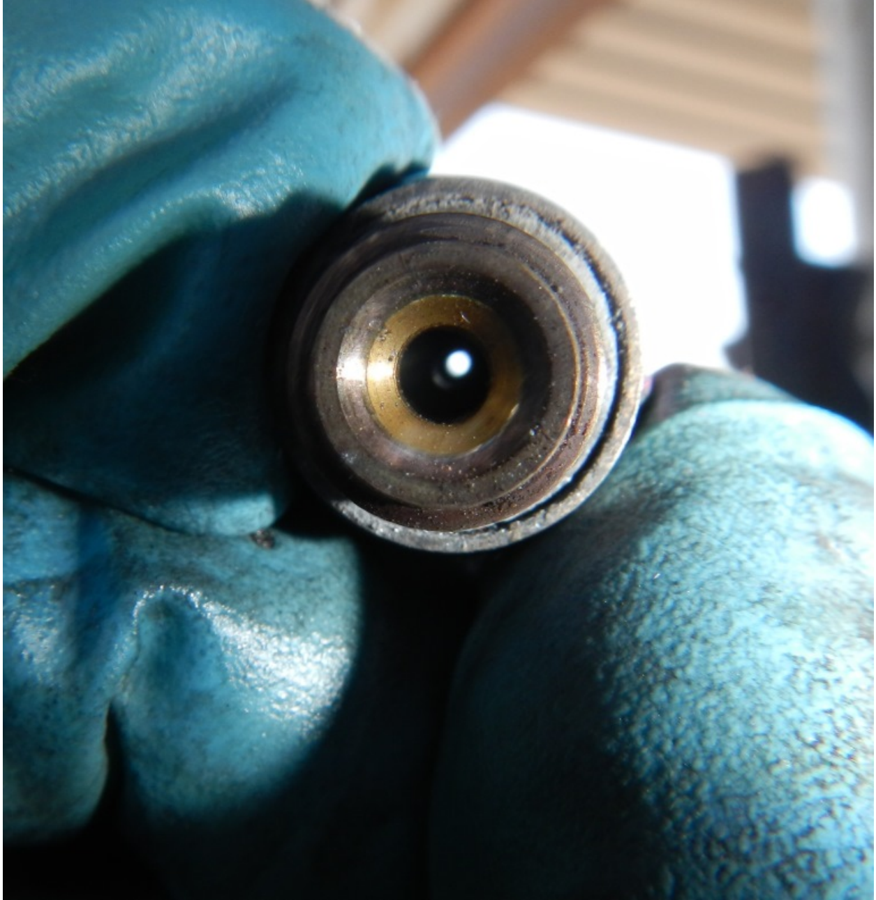
Figure 43 - Exemplar Nozzle (note clear orifice)
