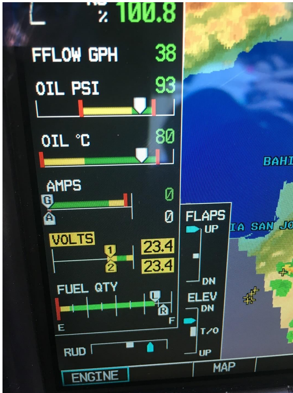
Figure 6. Photo taken at 23:11:46 UTC of a portion of the MFD screen indicating bus 1 and 2 voltages at 23.4V and flaps up.
