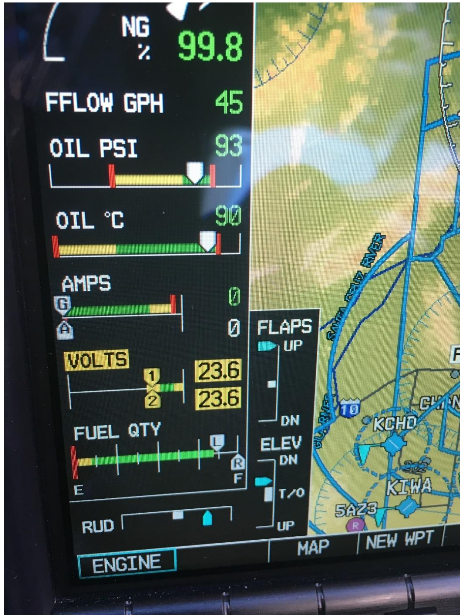
Figure 5. Photo taken at 23:03:26 UTC of a portion of the MFD screen indicating bus 1 and 2 voltages at 23.6V and flaps up.
