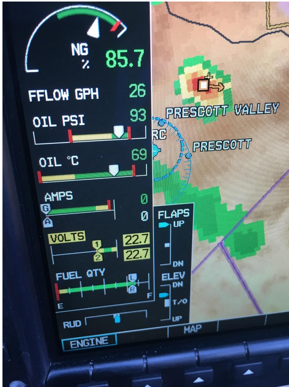
Figure 8. Photo taken at 23:27:21 UTC of a portion of the MFD screen indicating bus 1 and 2 voltages at 22.7V and flaps up.
