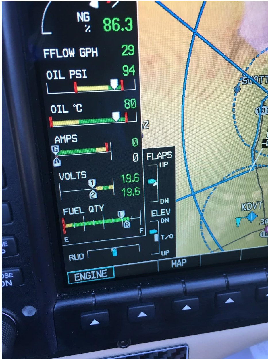
Figure 9. Photo taken at 23:41:12 UTC of a portion of the MFD screen indicating bus 1 and 2 voltages at 19.6V and flaps.
