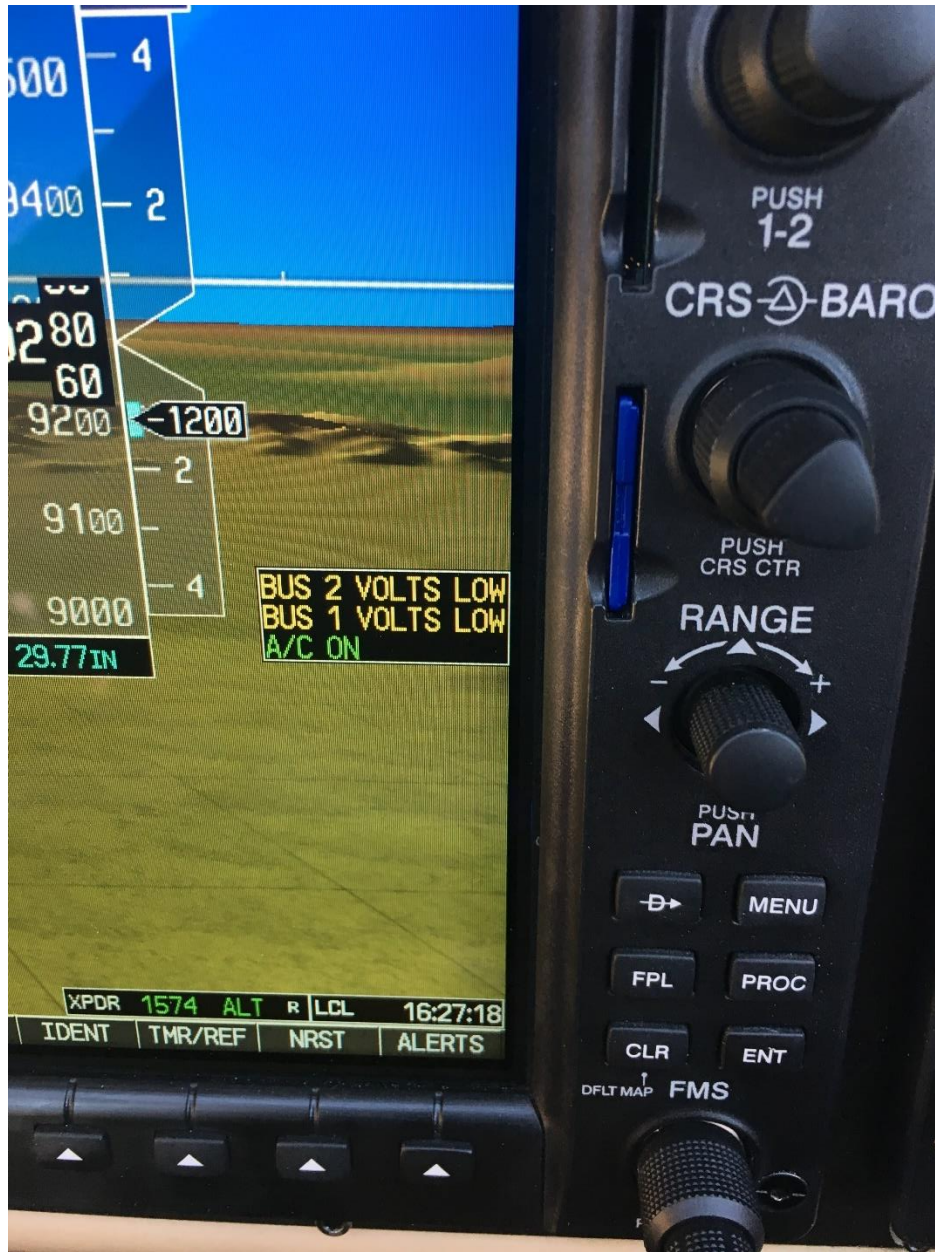
Figure 7. Photo taken at 23:27:18 UTC of a portion of the PFD screen indicating bus 1 and 2 voltages “LOW” and “A/C ON.”
