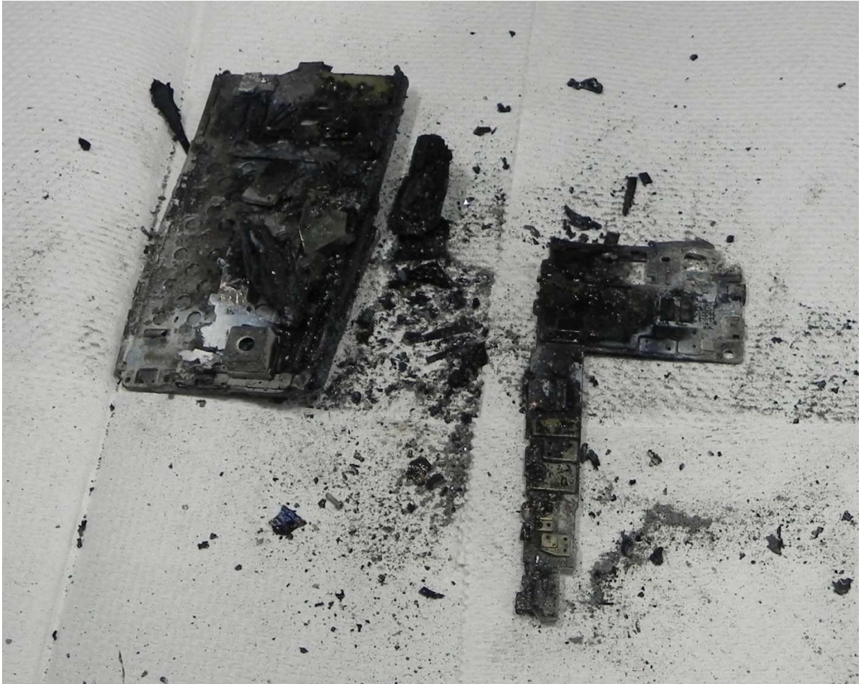
Figure 2. Remains of a smart-phone device showing severe fire damage.
