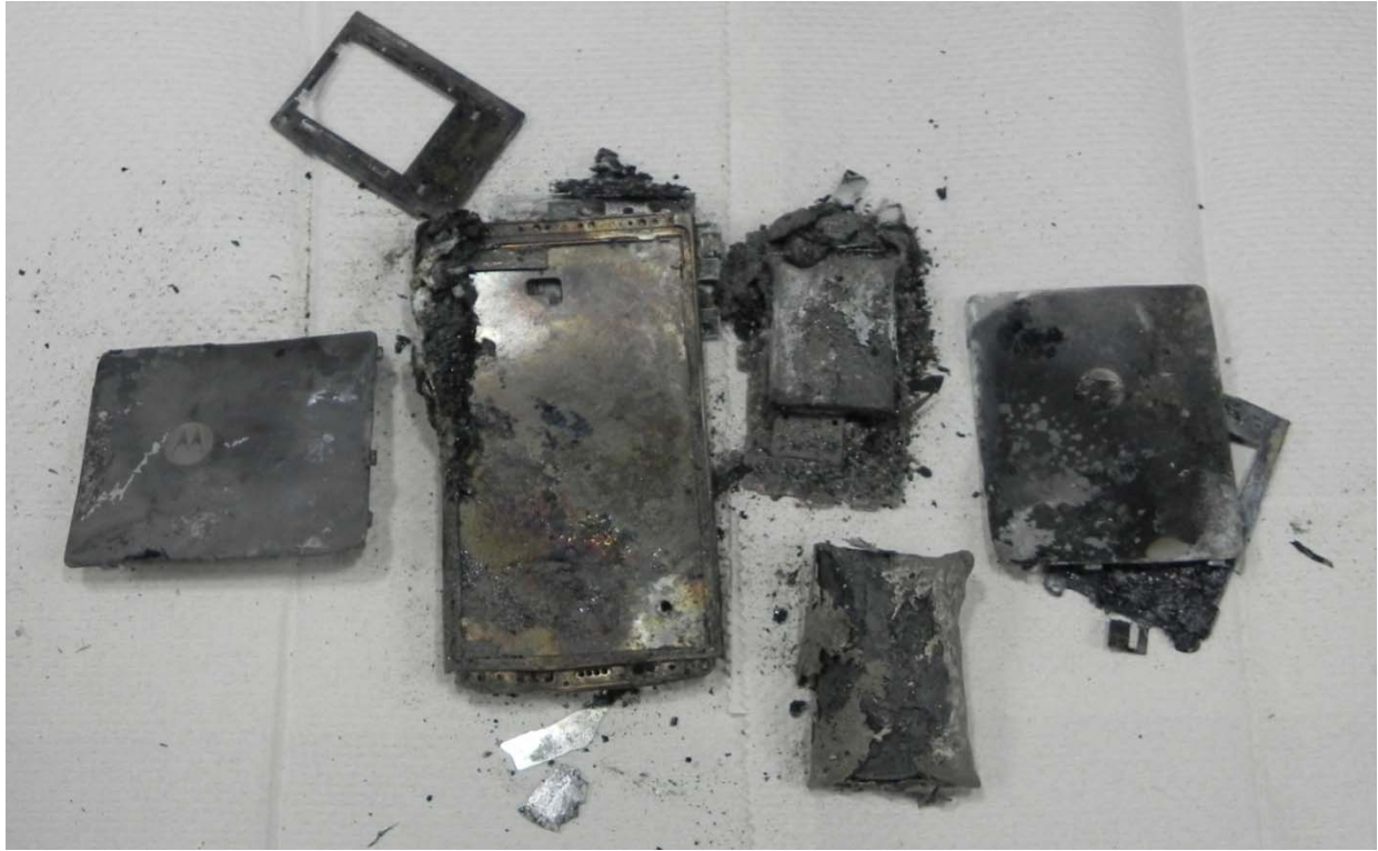
Figure 1. Remains of several smart-phone devices showing severe fire damage. One part shows traces of the Motorola logo.
