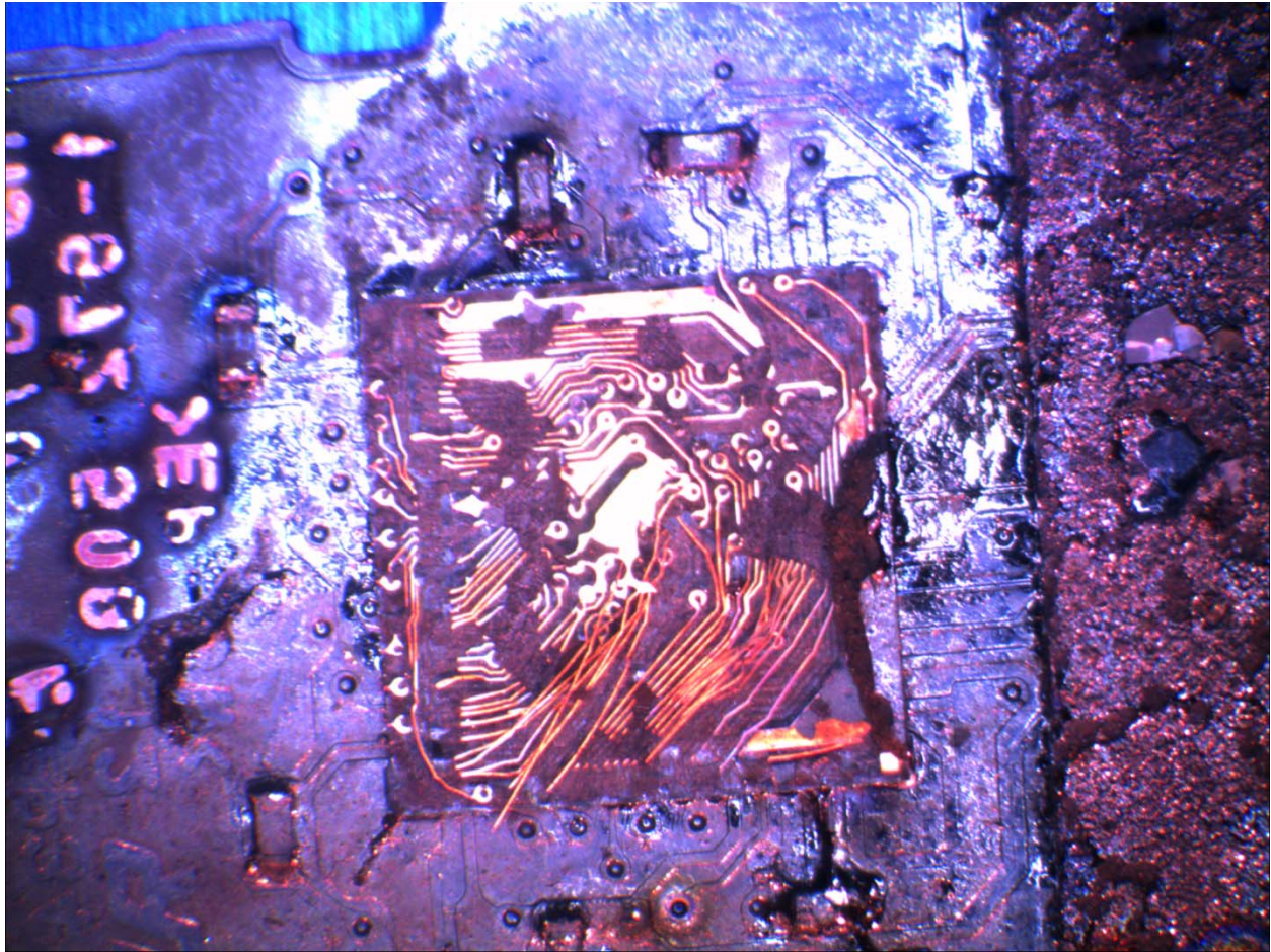
Figure 5. Internal view the of memory–stick controller integrated circuit from a Sony Cybershot 10.1 mega-pixel digital camera showing destruction due to fire.
