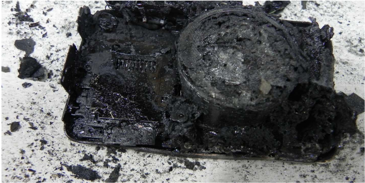
Figure 3. Remains of Sony Cybershot 10.1 mega-pixel digital camera showing severe fire damage.
