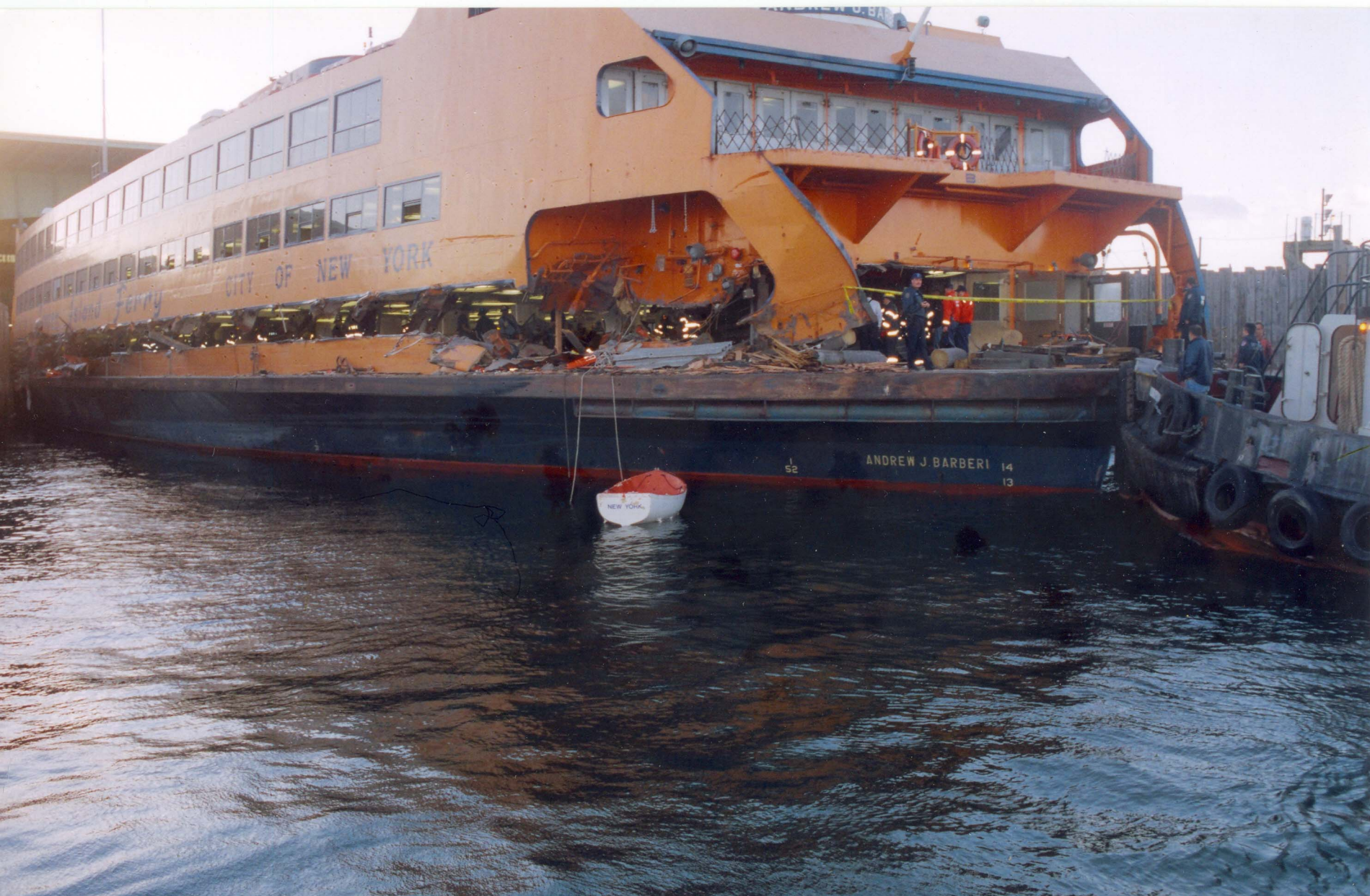
NYPD Photo of Vessel Damage Exterior
