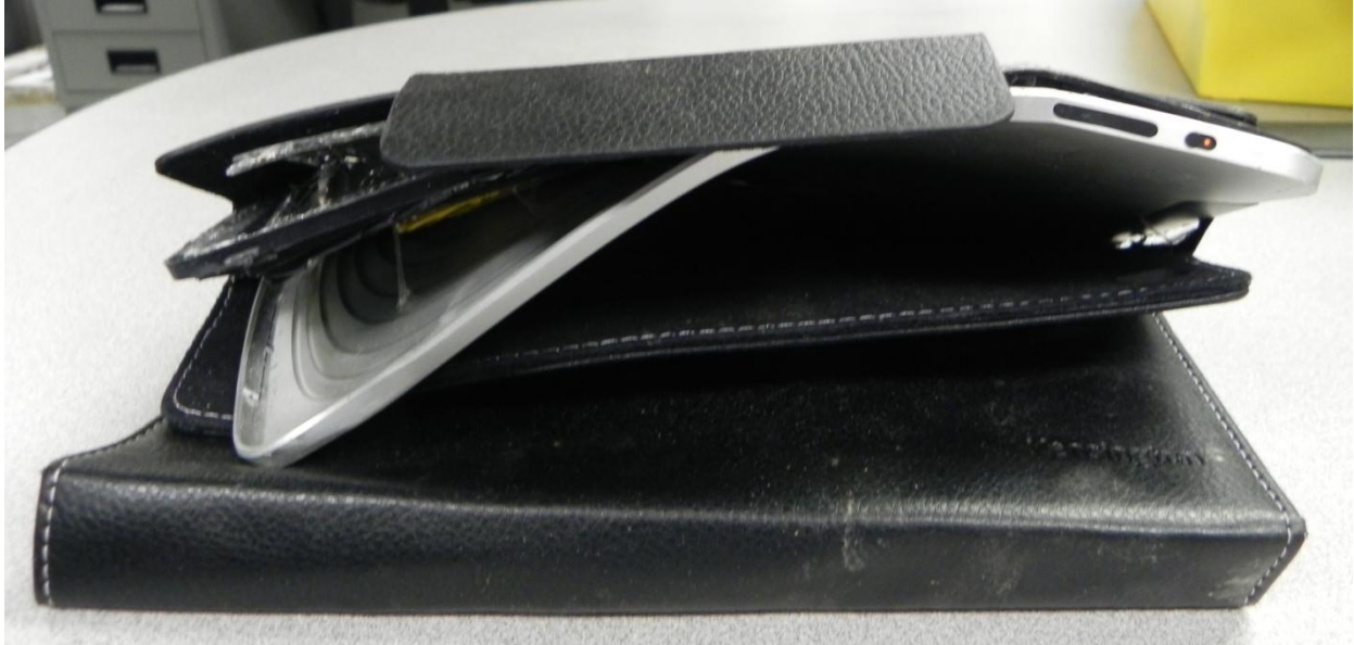
Figure 2. External side view of the Apple iPad (GB044RN6ETV) showing impact damage and severe deformation to the aluminum outer shell. The main printed circuit board (PCB) is located to the right in the image.
