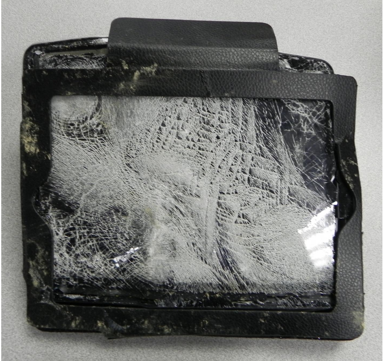
Figure 1. External front view of the Apple iPad (GB044RN6ETV) showing impact damage to the touchscreen.
