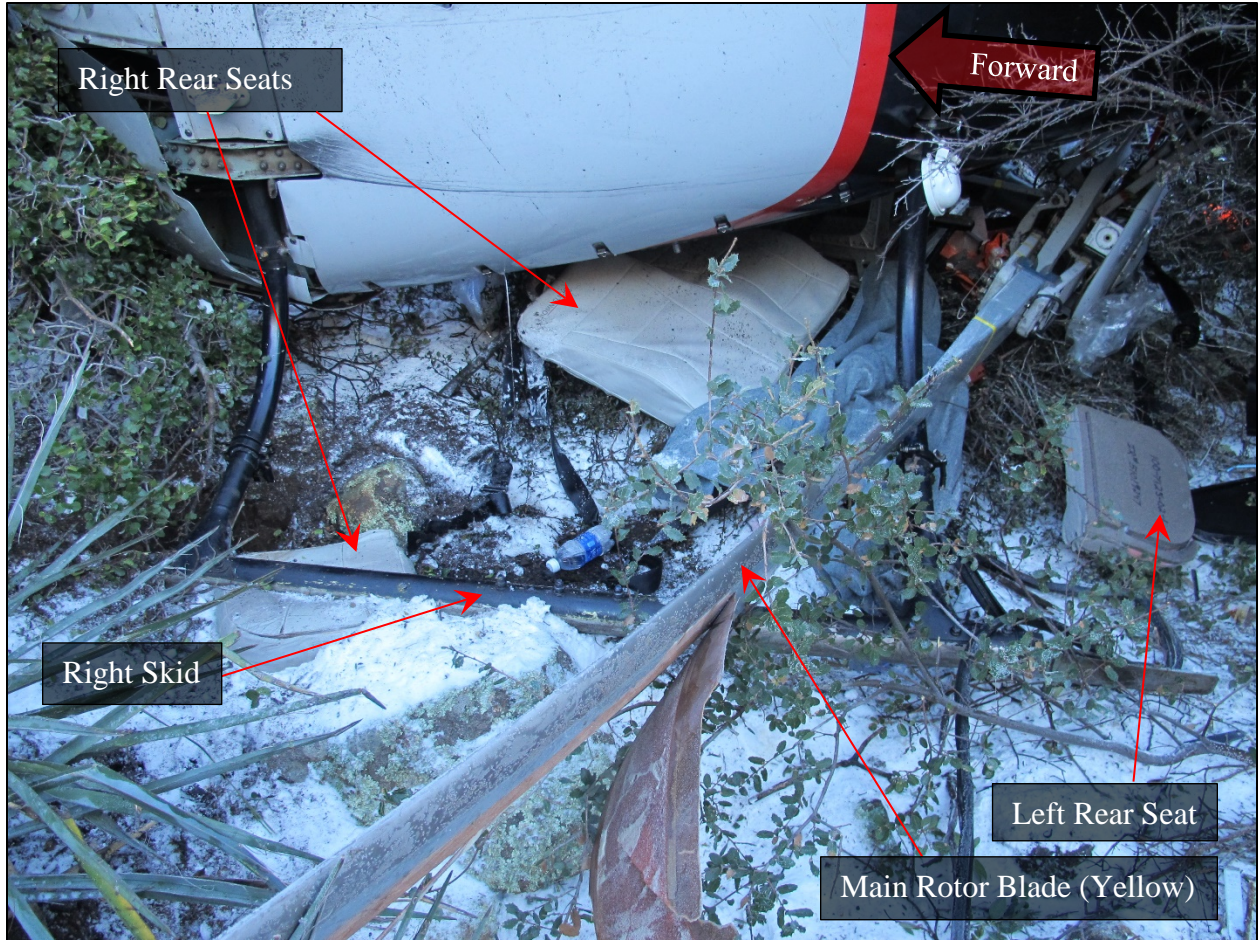
Figure 5-Main Wreckage, Looking Upslope, Southeast
