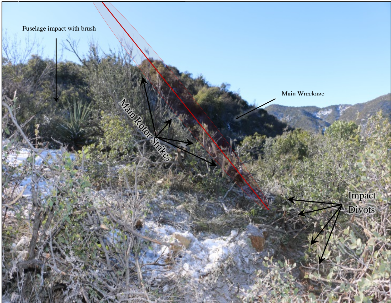
Figure 2-First Identified Point of Contact (FIPC)
