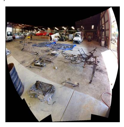
The forward seat had thermal damage. The rear seat revealed impact damage to its structure and deformation of the metal lower seat webbing.
