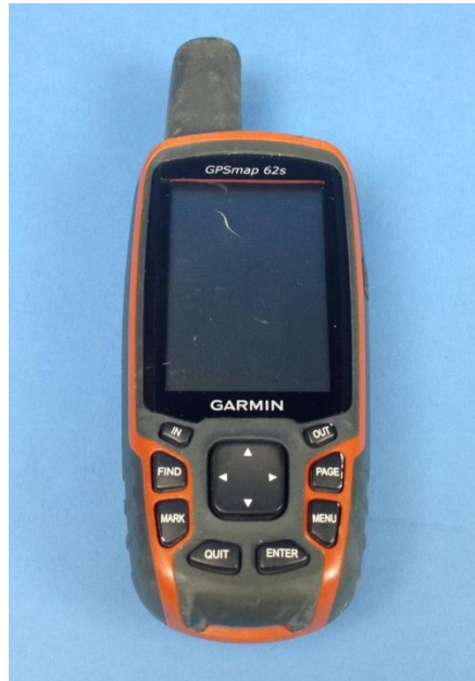
Figure 1. The arrival condition of the Garmin GPSMAP 62s.
