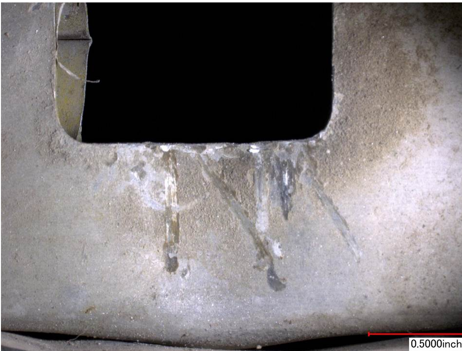
Photo 10 - Detailed view of scrape marks on aft side of elevator spar. View looking forward.
