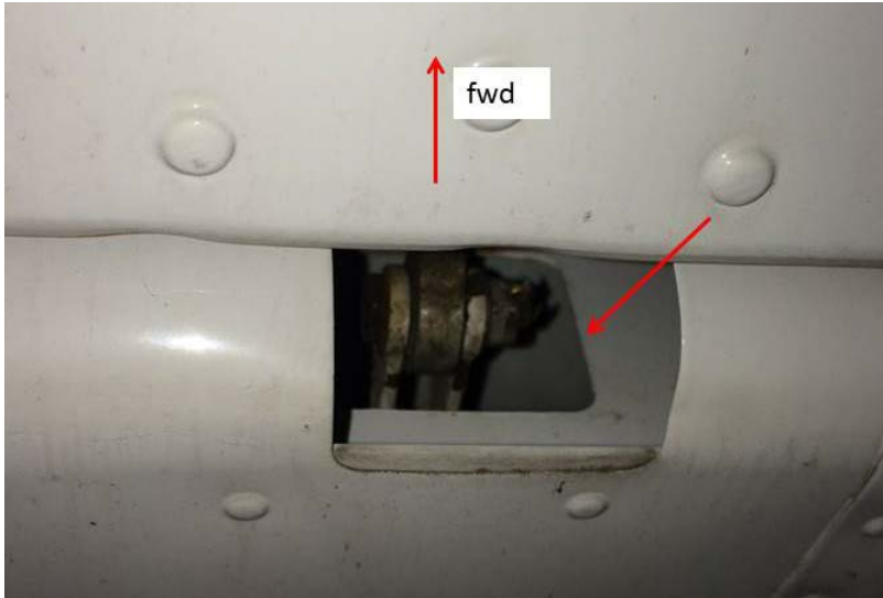
Photo 15 - Another C310. View looking up and aft. The trim actuator was fully extended (AND trim). The bolt through the rod-end bearing and fork is near the elevator spar.
