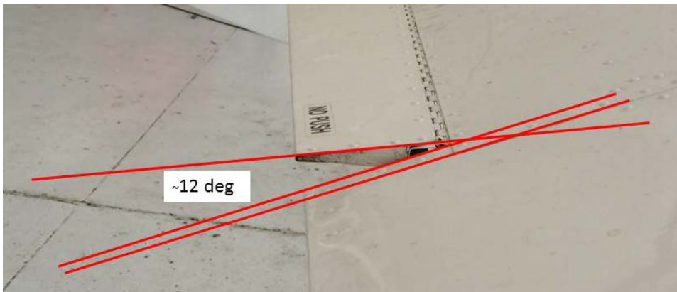
Photo 16 - Another C310. The tab TEU or actuator AND trim position, about 12 degrees.
