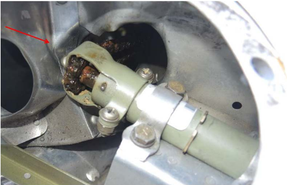
Photo 3 - Trim tab actuator. The actuator had been impacted from the front (see arrow).
