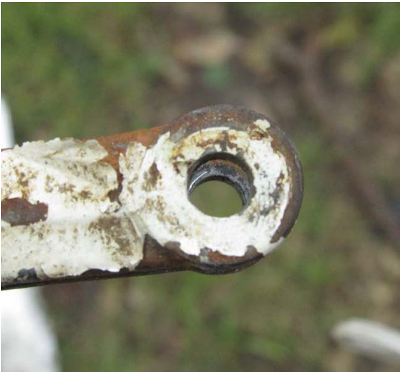
Photo 5 - Forward end of the pushrod. There was no apparent damage to the bolt hole (side two).
