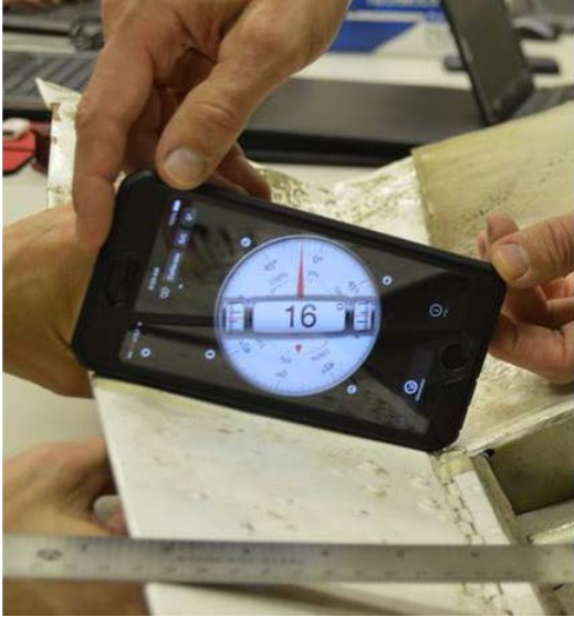
Photo 21 – Slope of tab. The tab deflection is about 39 degrees.
