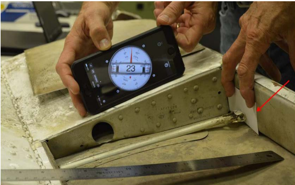
Photo 20- Slope of elevator. The pushrod was positioned as if the elevator spar had not been bent. The white paper replicates an unbent spar.
