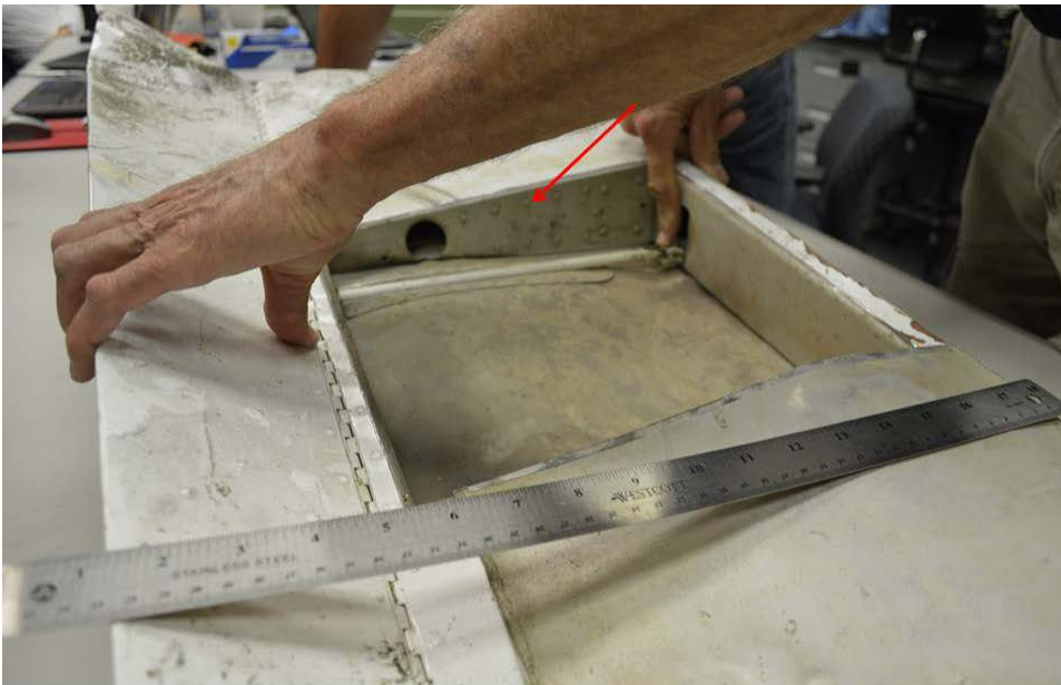
Photo 8 – The clevis fork is placed behind the elevator spar. The tab is deflected up to pull the fork aft, well past the limits of normal travel.
