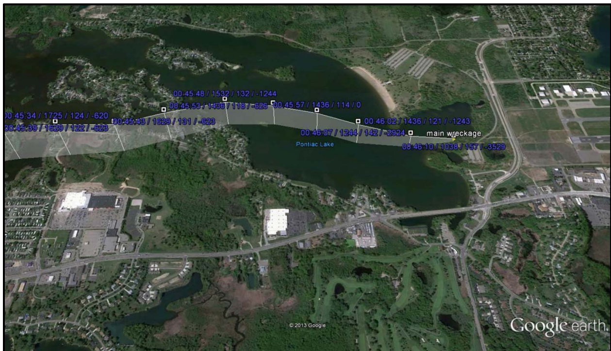
Figure 3: Final approach into KPTK with hh:mm:ss / hmsl (ft) / Vc (kt) / ROC (fpm)
