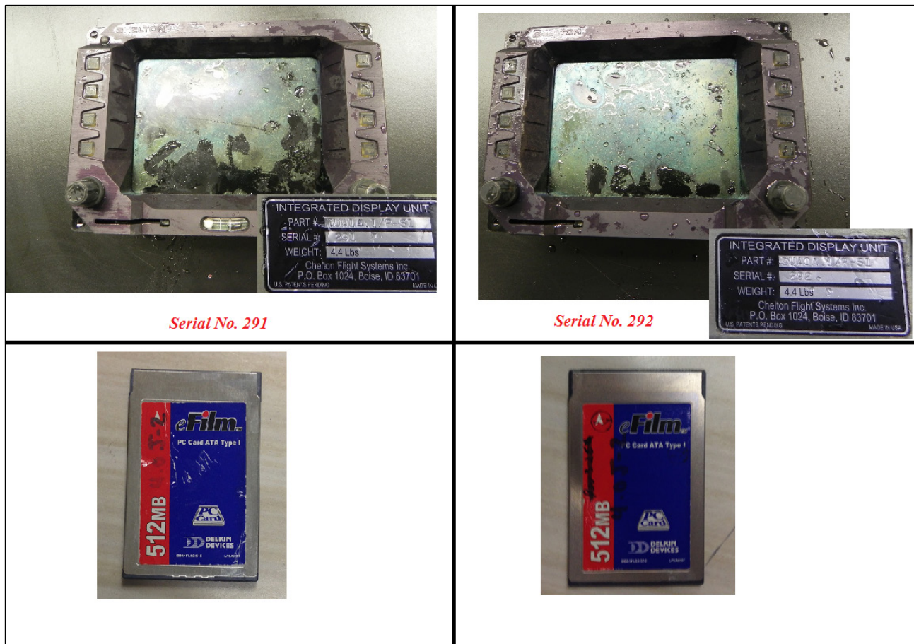
Figure 3. Damaged exterior of Chelton Flight Systems IDUs.
