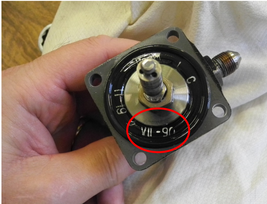
Membrane with Manufacture Date of July 1990 – Undamaged
