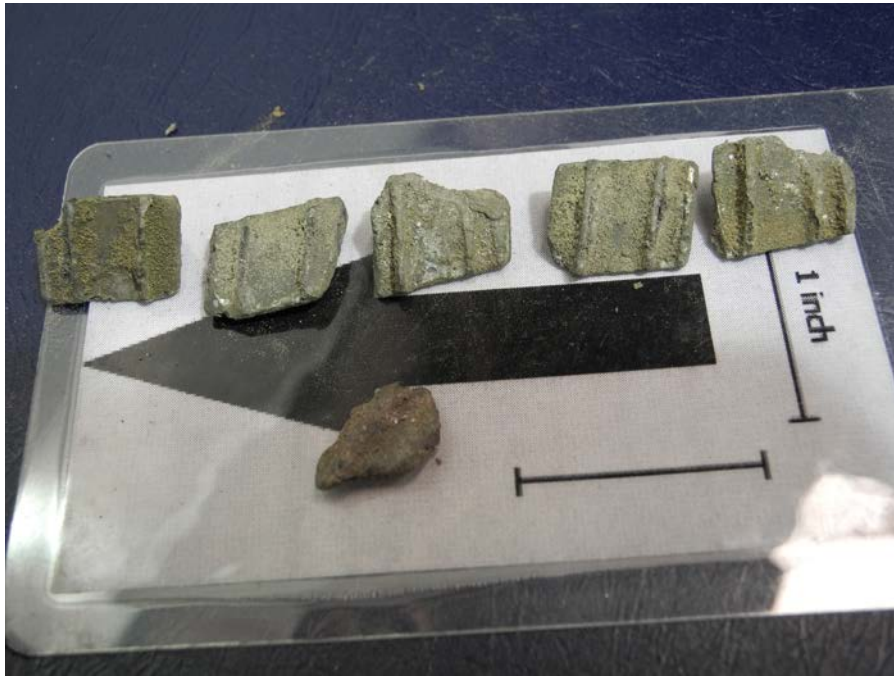
Fractured Blade Tip Segments Found in Exhaust Duct
