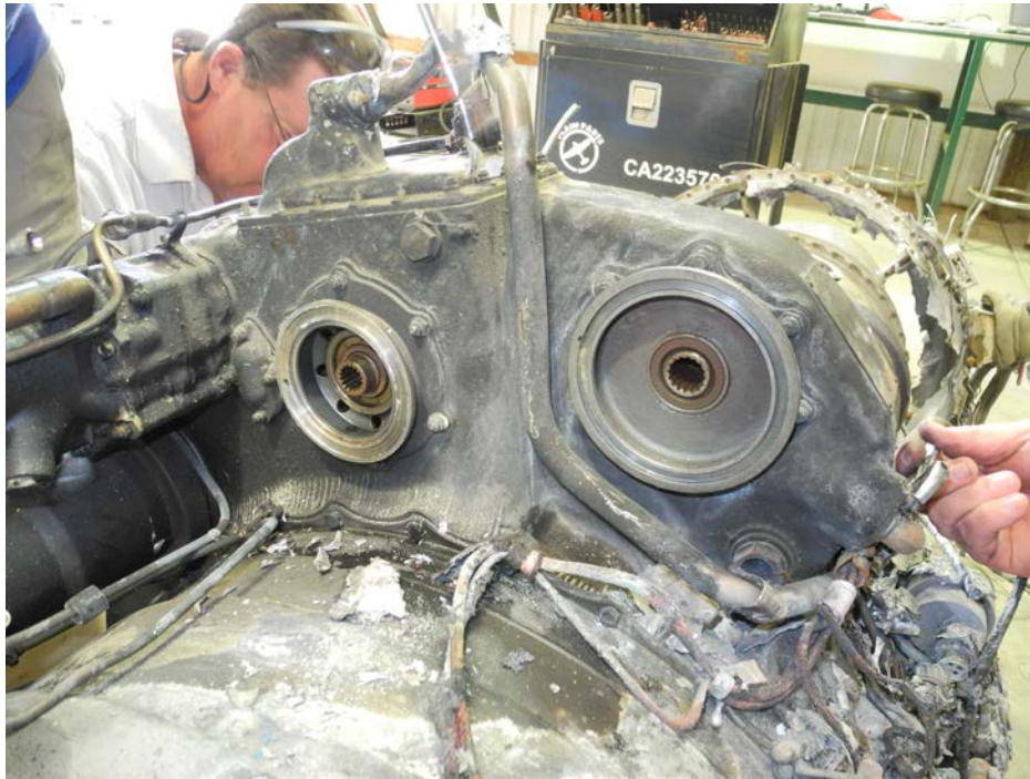
Accessory Gearbox - Front View - Splines Undamaged
