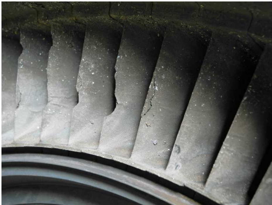
2 nd Stage (1 st Stage LP) Turbine Nozzle – Trailing Edge Fracture Details
