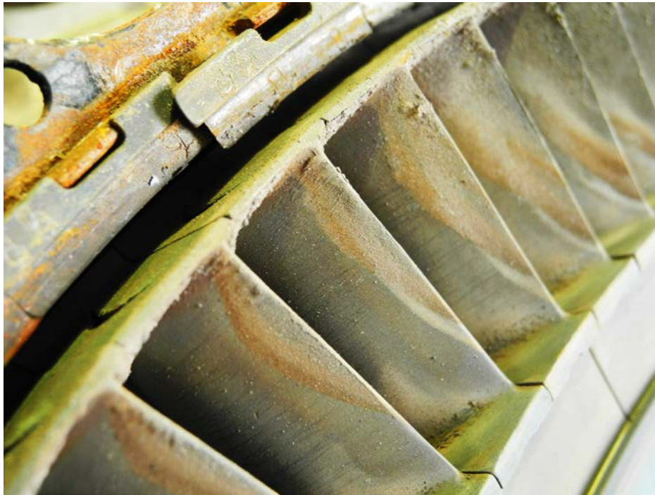
HP Turbine - Details of Streaking Marks
