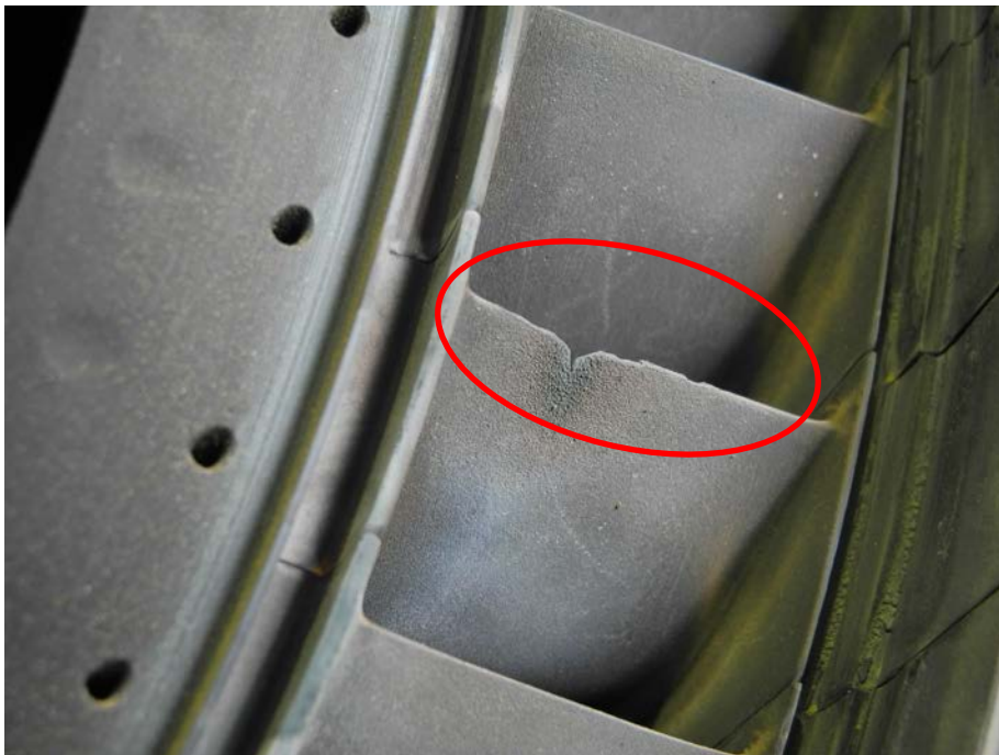
Details of Eroded HP Turbine Nozzle Vane Trailing Edge
