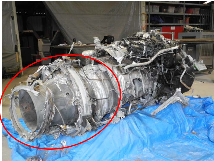
HP Compressor, Combustor & Turbine Housings and Exhaust Pipe
