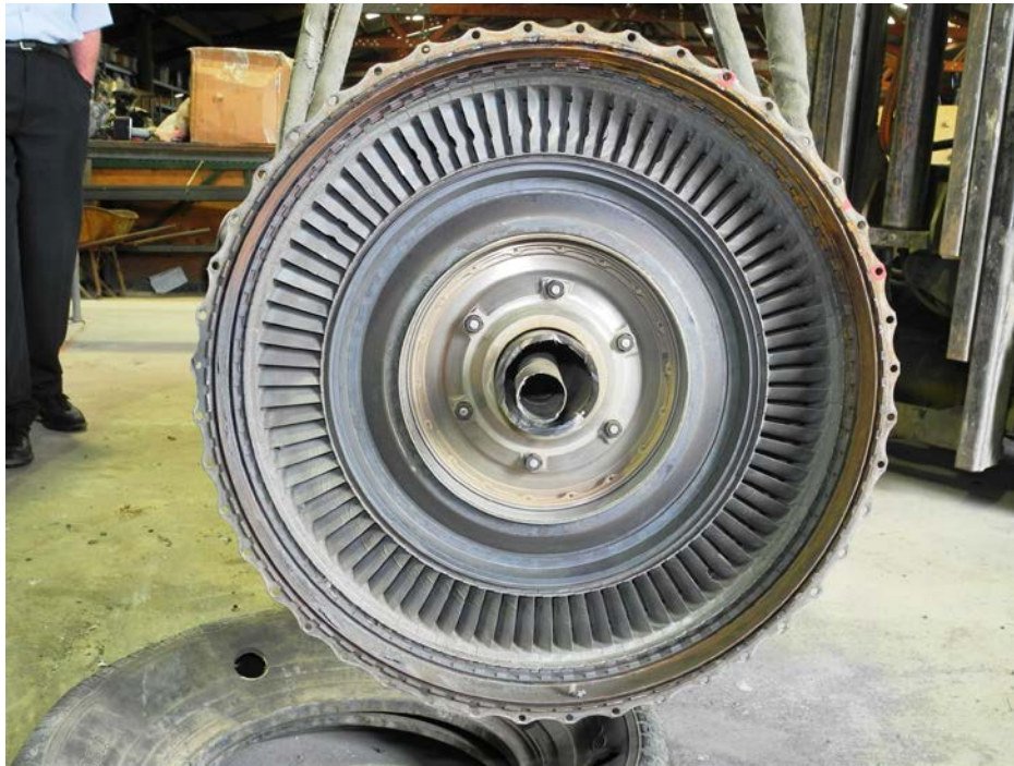
2 nd Stage (1 st Stage LP) Turbine Nozzle – In Situ - Aft View
