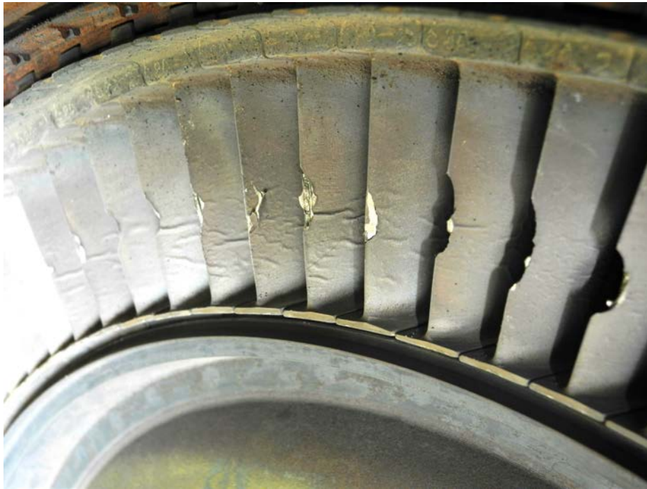
2 nd stage (1 st Stage LP) Turbine Nozzle – Surface Rippling Details
