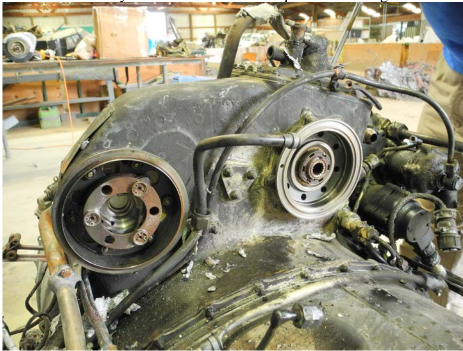
Accessory Gearbox – Aft View - Splines Undamaged.
