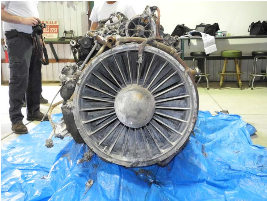
Front View - LP Compressor Inlet Guide Vane Assembly
