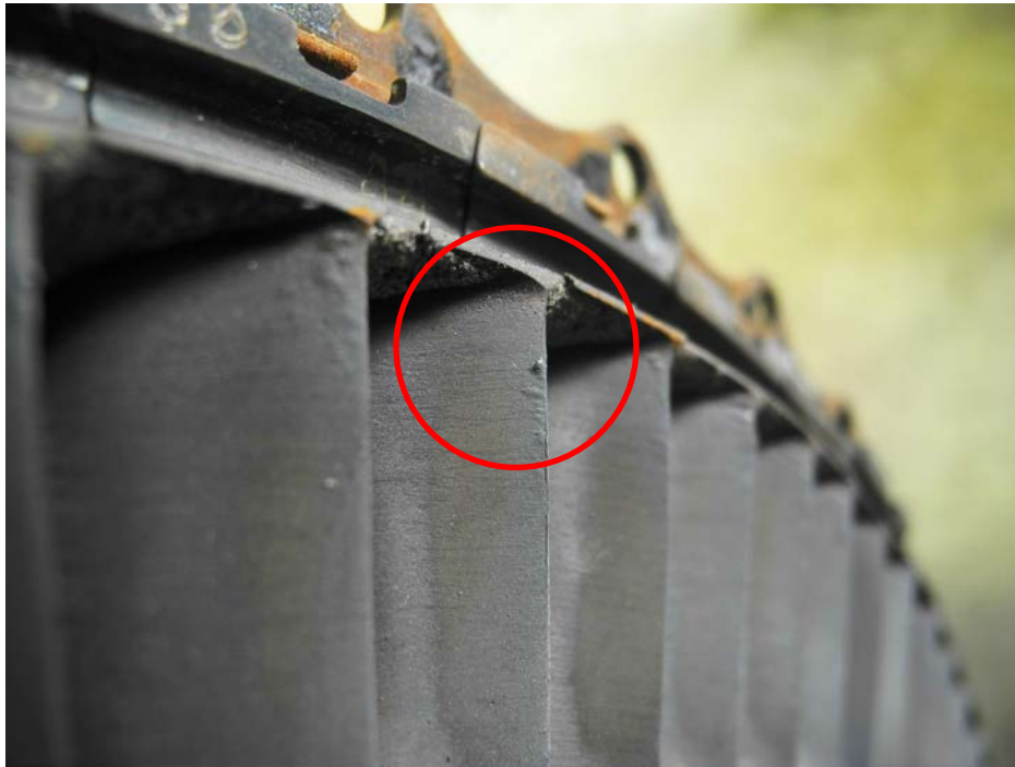
HP Turbine Blades - Concave Side Trailing Edge Rippling
