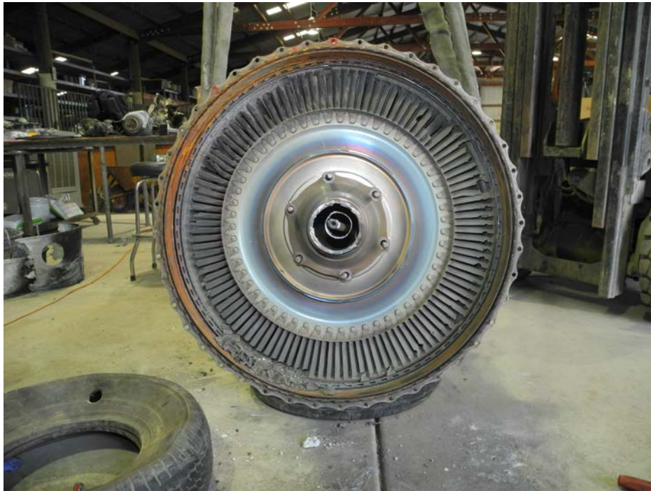
2 nd Stage (1 st Stage LP) Turbine – In Situ – ALF
