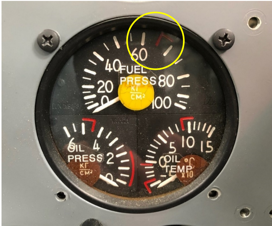
Figure 6 – Exemplar 3-in-1 Gauge in Cockpit – Note Fuel Pressure Redline of 65 Atmospheres
