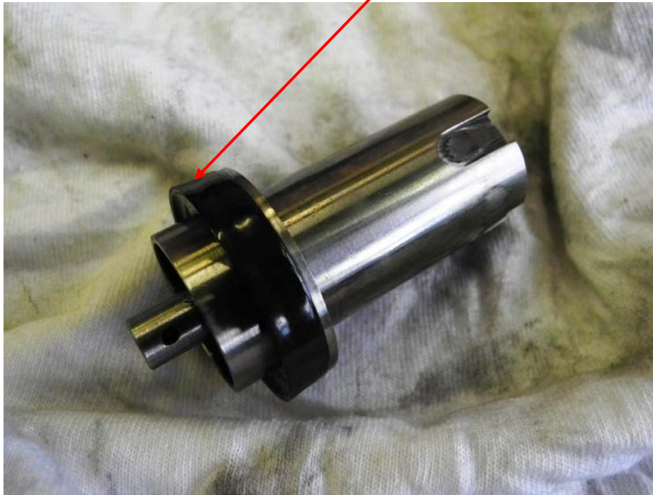
Shuttle Valve – Slightly Worn Sliding Seal
