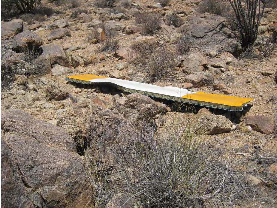
Photo 4 FAA Photo First Identified Debris - Outboard Piece of Main Rotor Blade Afterbody
