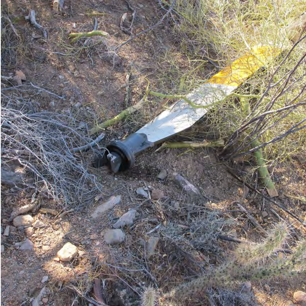
Photo 9 Robinson Photo of Separated Main Rotor Blade Hub End
