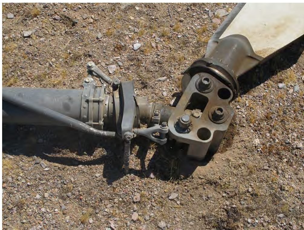
Photo 13 Bent Main Rotor Driveshaft
