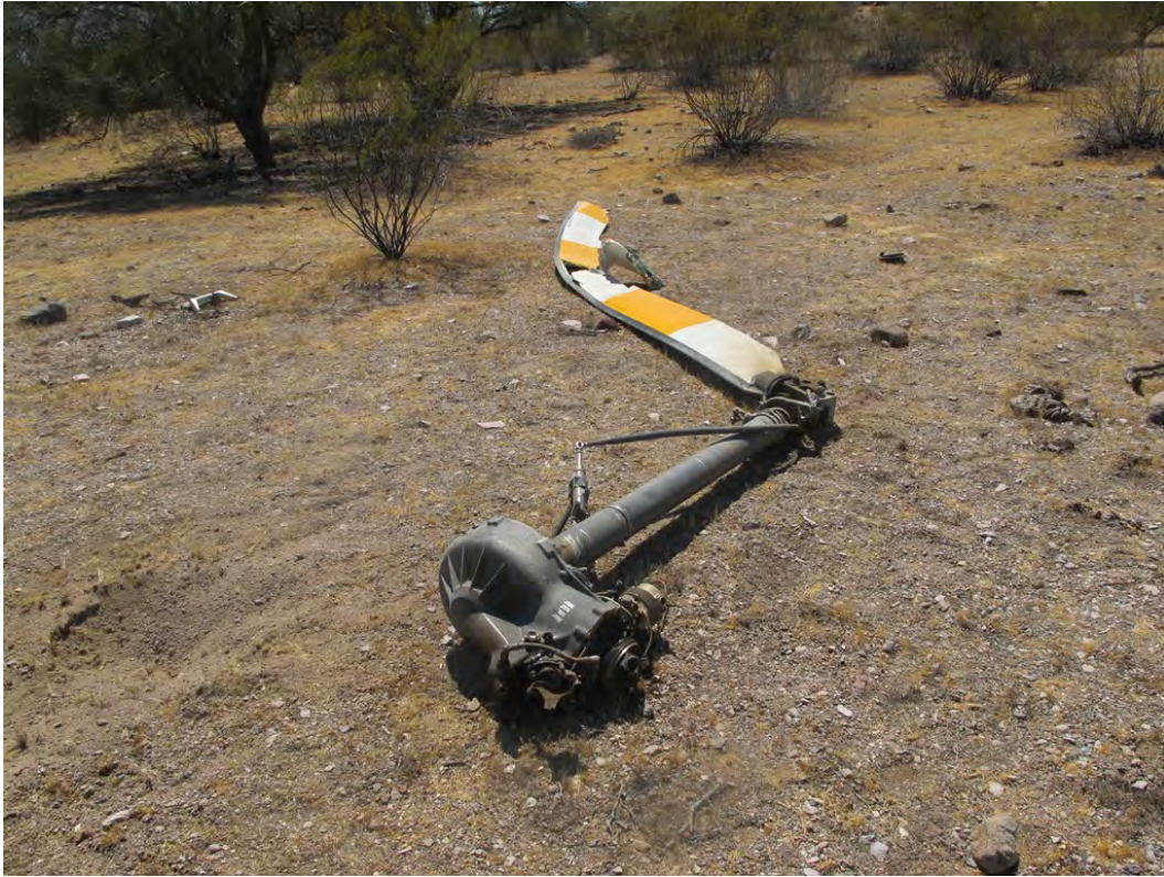
Photo 14 Main Rotor Gearbox, Mast, and Main Rotor Blade
