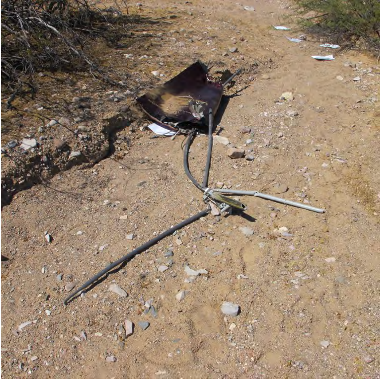
Photo 7 Robinson Photo of Mast Fairing with Main Rotor Flight Controls
