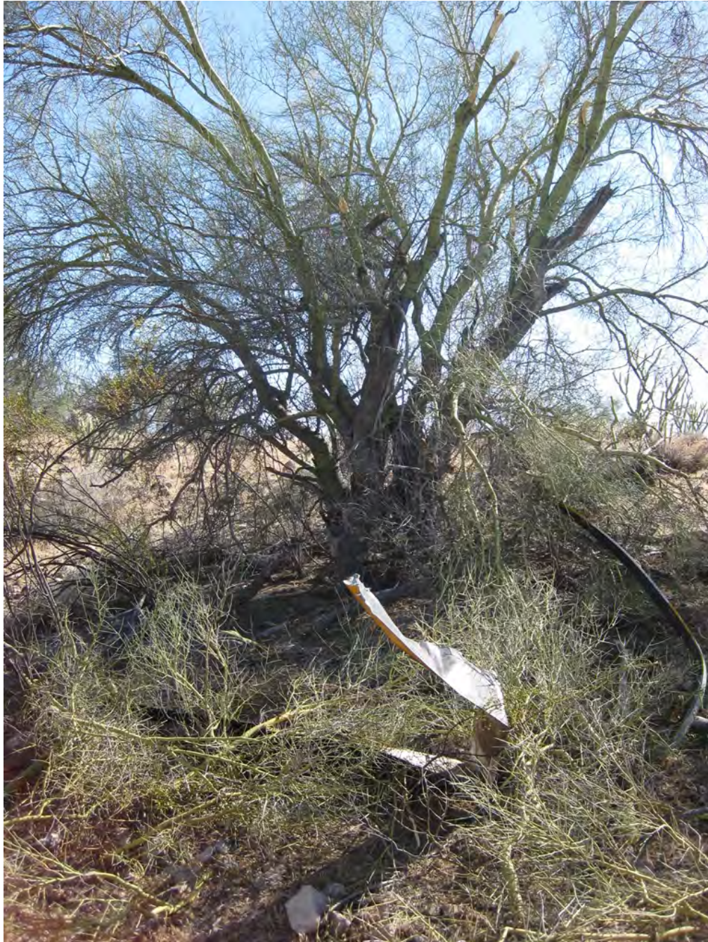
Photo 8 FAA Photo Separated Main Rotor Blade
