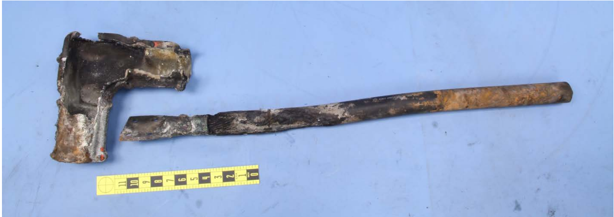
Figure 1: Portions of pig tail cable and cable connector cover as received.
