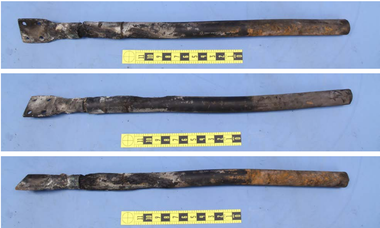
Figure 2: Portion of the pig tail cable (3 views).
