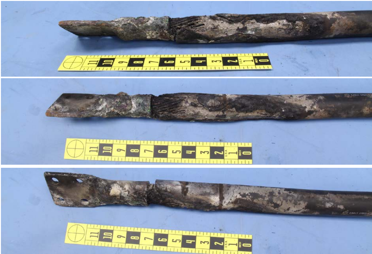
Figure 3: Close up of damage to the lug end (3 views).
