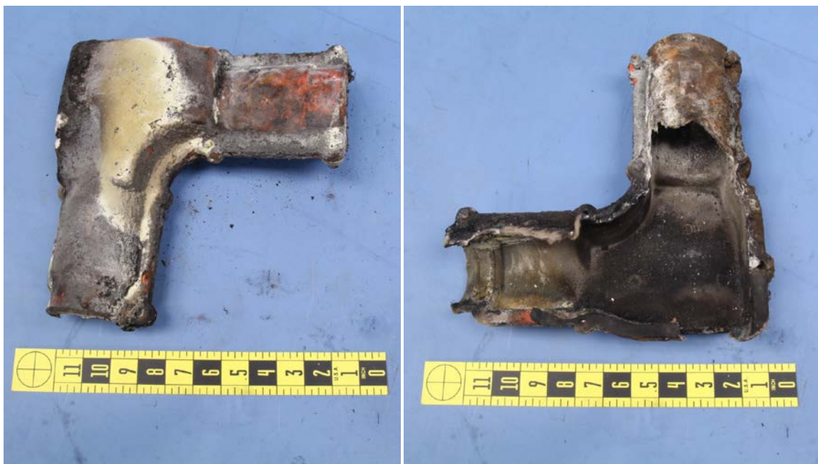
Figure 4: Damaged cable connector cover ("boot").
