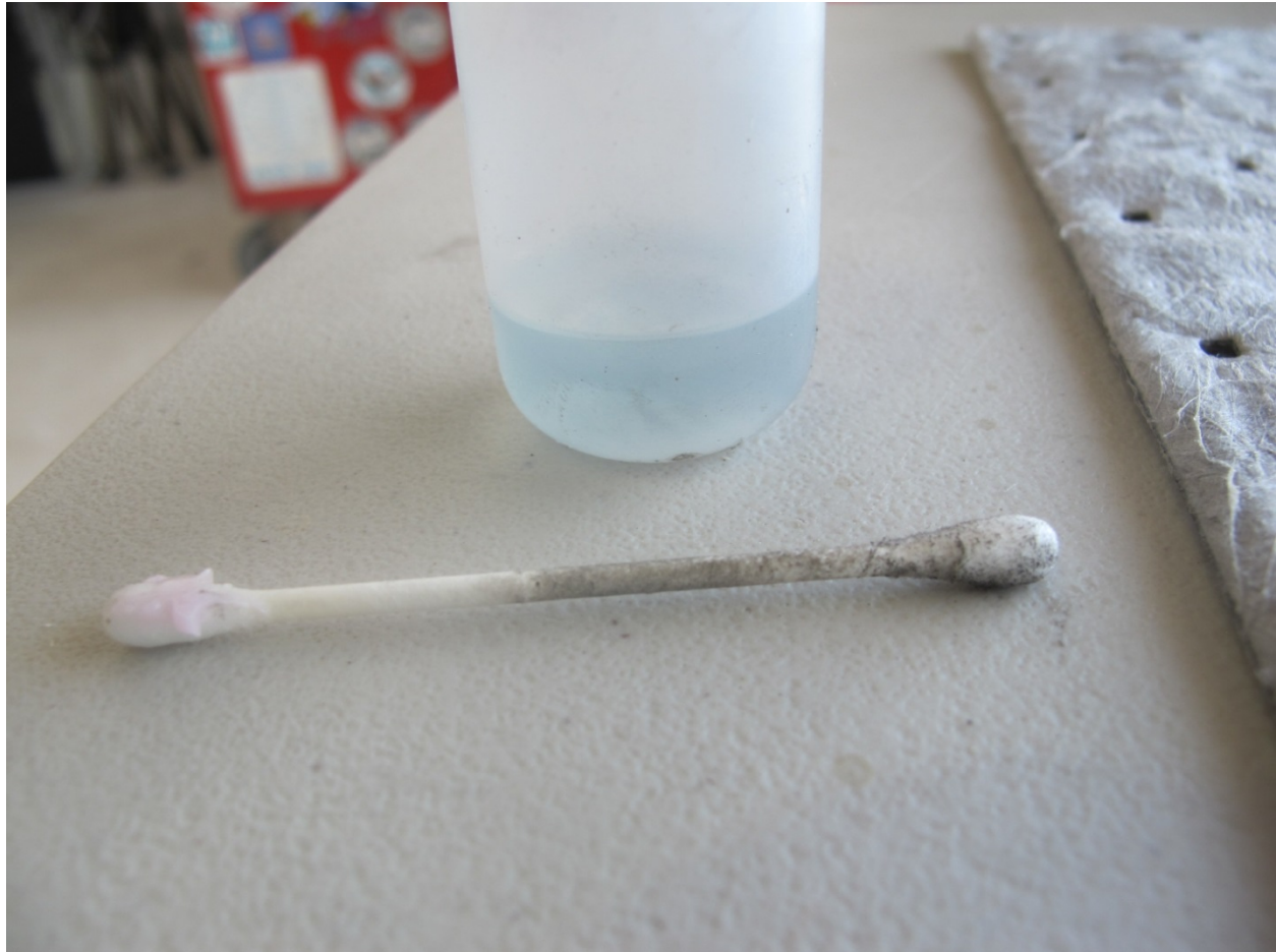
Photo 3 Water Paste Test of Fluid from Gascolator
