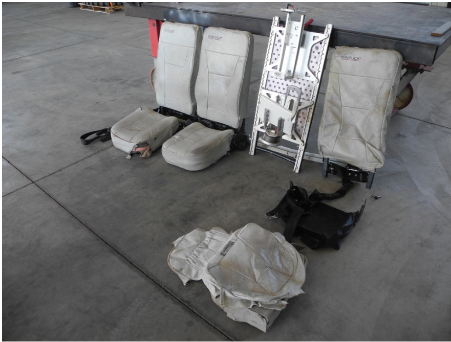
Photo 9. Reconstruction of the three seats and cargo pallet.
