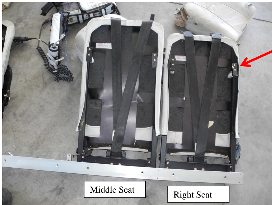
Photo 6. A view of the rear of the middle and right seat backs installed on the lower lateral track. The unlabeled arrow points to the deformation on the right hook of the right seat.
