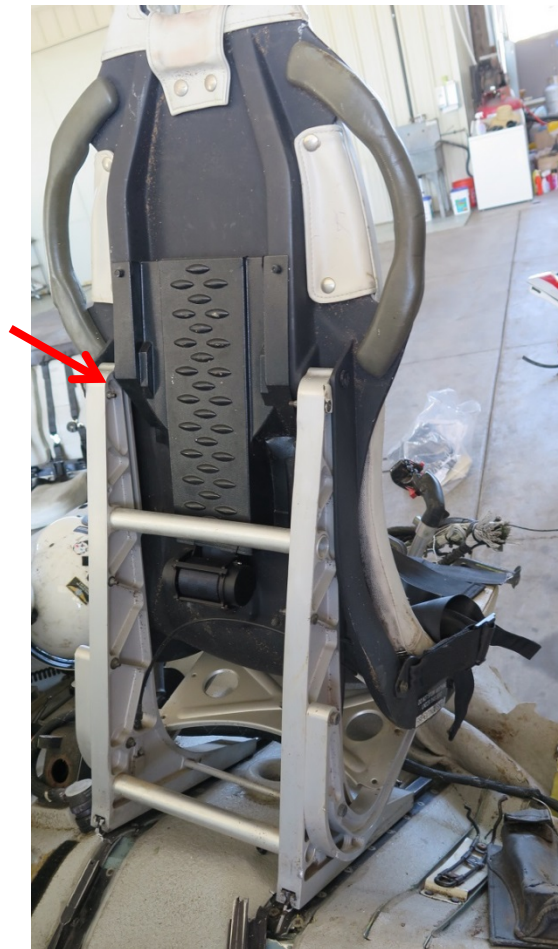
Photo 3. The pilot seat mounted to the floor tracks. The unlabeled arrow points to the seat stroking track. (Photo courtesy of Airbus Helicopters)
