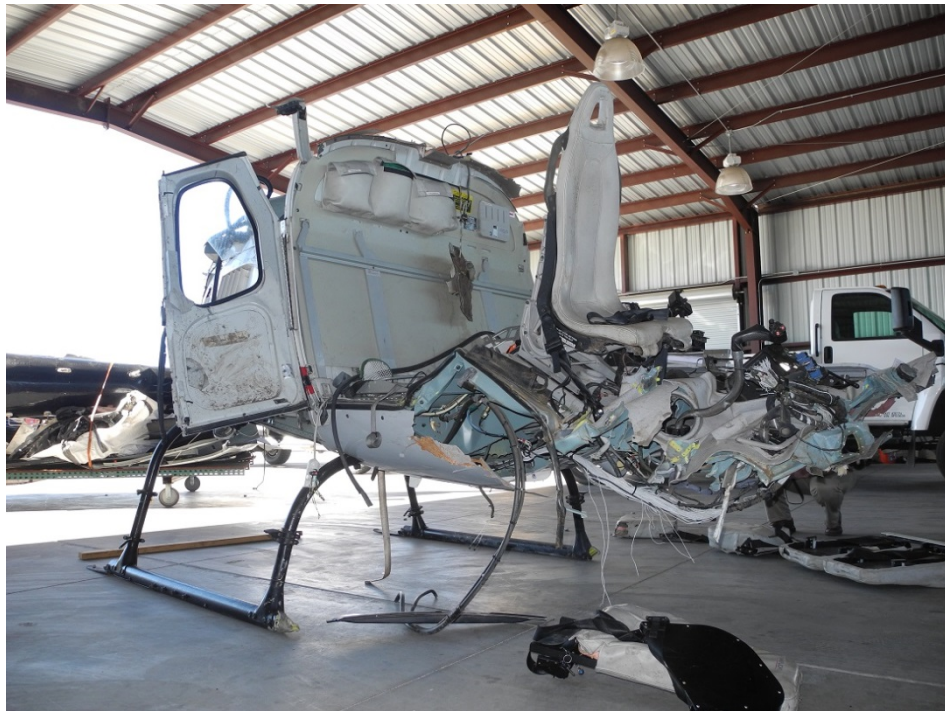
Photo 2. The pilot seat and cabin floor buckling.
