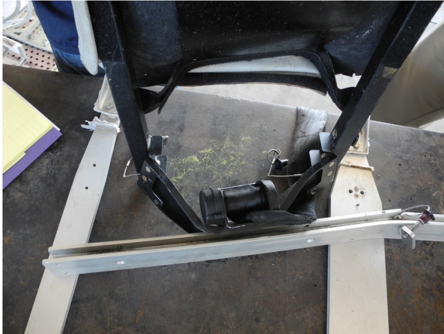
Photo 7. Rear left seat lower mounting plate deformation.
