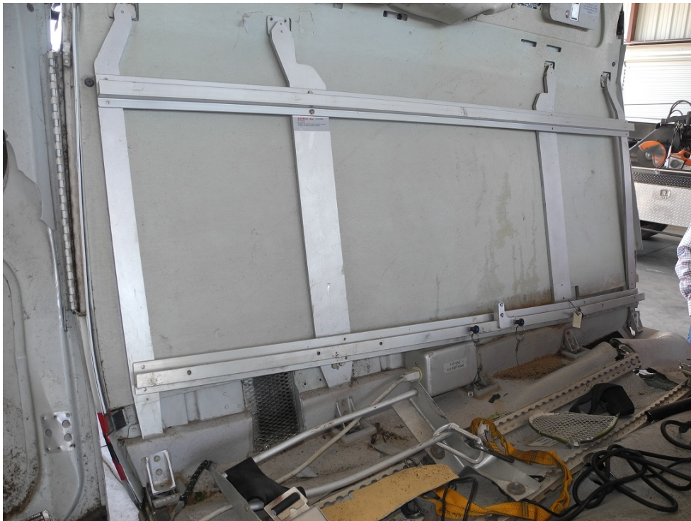
Photo 4. A reconstructed assembly of the lateral tracks and vertical straps.
