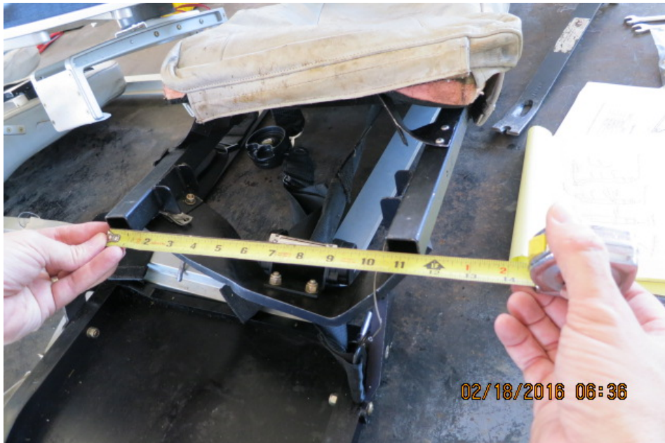
Photo 8. Measurement of the lower seat back frame deformation for the rear left seat. (Photo courtesy of Air Methods)
