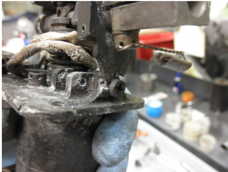
Photo No. 12: Close up view of base of manual lever arm spindle support broken on right side.
