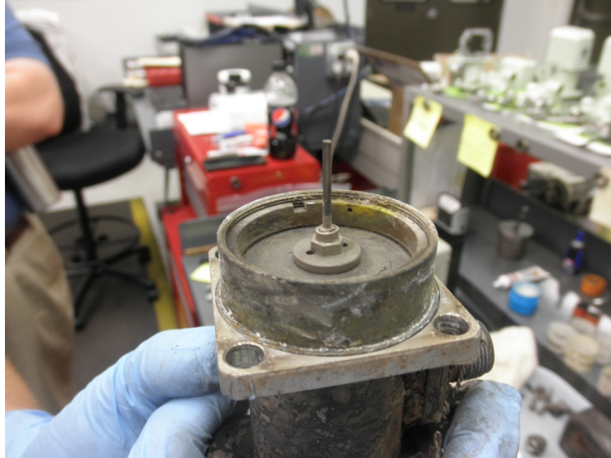
Photo No. 8: View of poppet stem showing it is a long stem and does not have the ball end.
