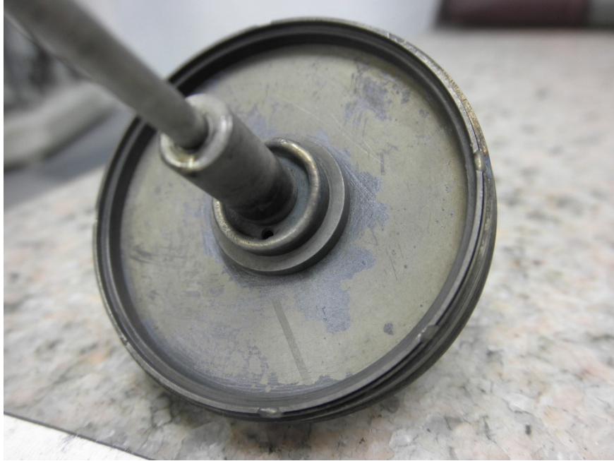
Photo No. 6: Close up of Belleville washer showing that it is intact.
