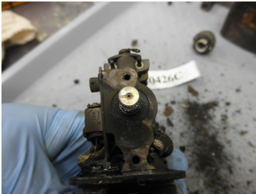
Photo No. 3: Close up of manual lever arm spindle with indexing line pointing to left.
