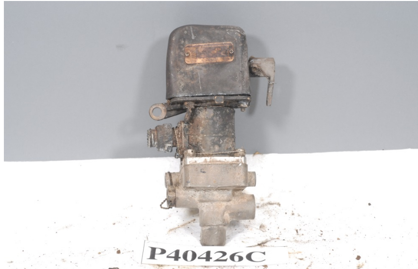
Photo No. 2: View of front of left engine's FSOV showing sooted body.
