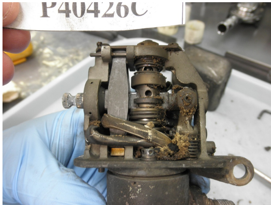
Photo No. 4: Close up of top of fuel shut off valve with cover removed showing fibrous material.
