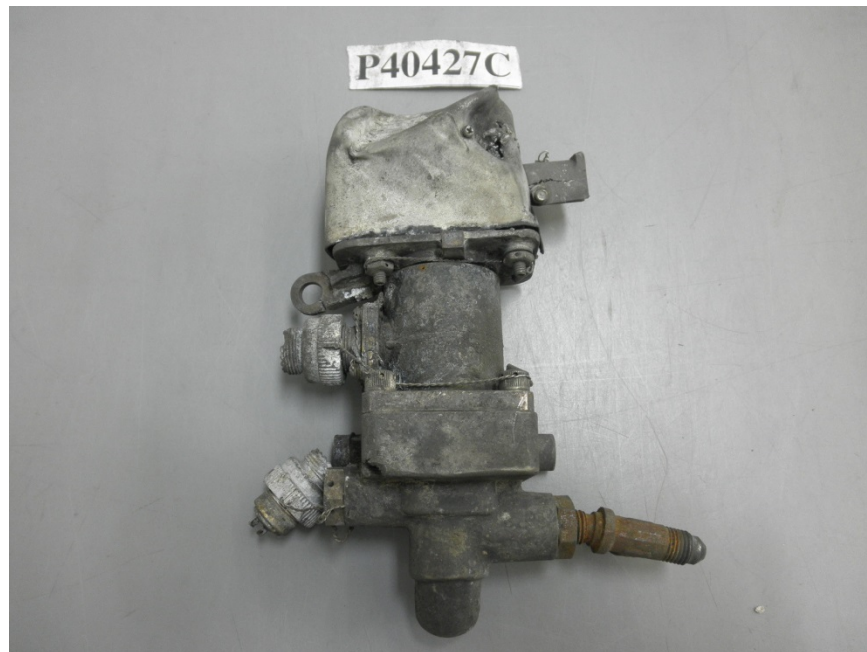
Photo No. 10: Left engine's FSOV showing body sooted and cover partially melted.
