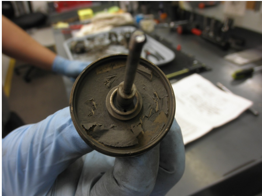
Photo No. 7: Close up of back side of Belleville washer showing coating peeling off.
