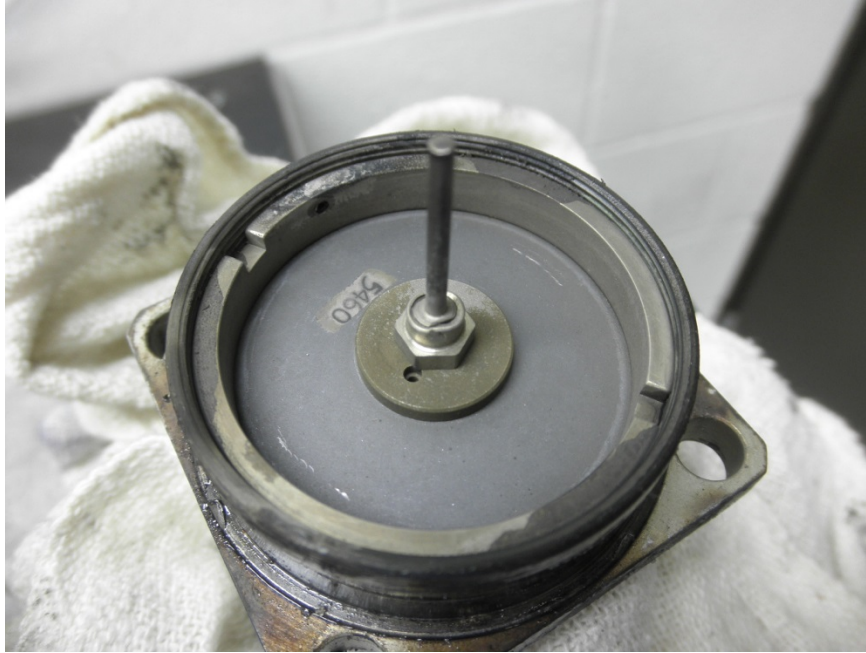
Photo No. 15: View of poppet stem showing it is a long stem and does not have the ball end.
