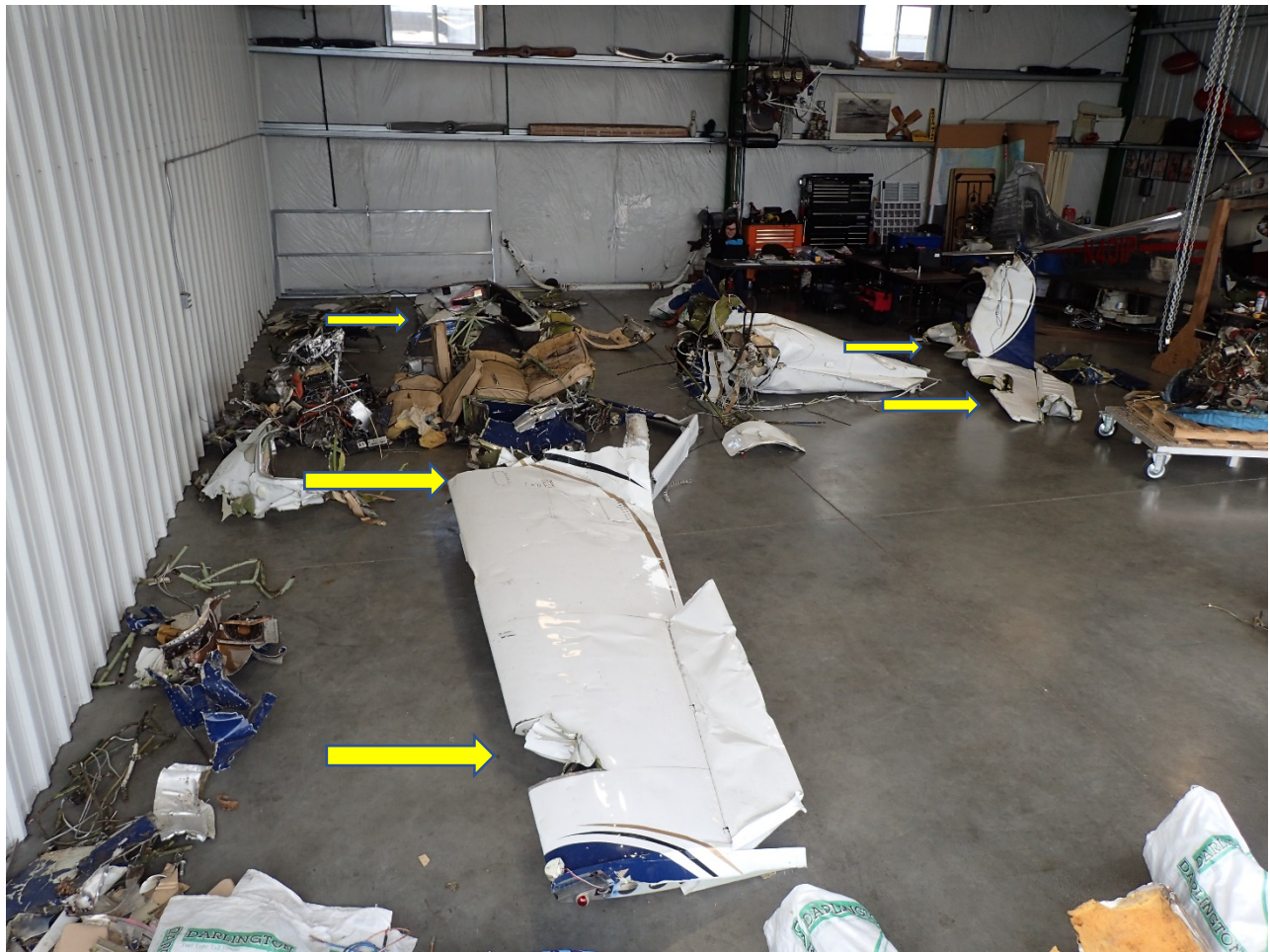
Figure 3. Wreckage at examination hangar with yellow pointers indicating tree strikes.
