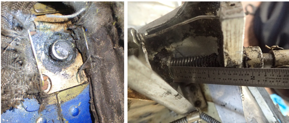
Figures 5. Fractured aft pitch trim jack screw (left) and Elevator Trim Assembly jack screw (right) indicating full nose down trim.
