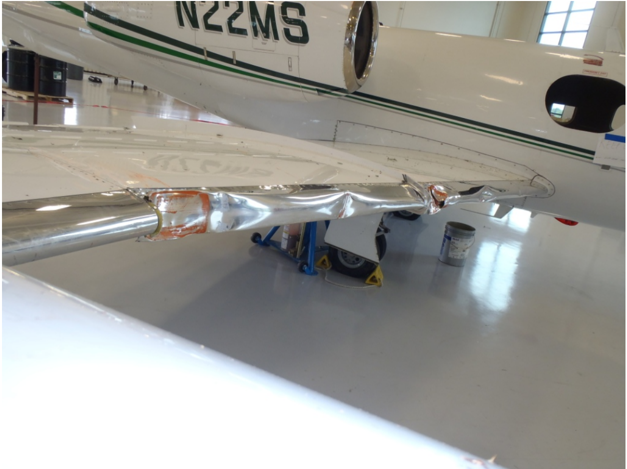
Photo 1 – Leading Edge Damage
