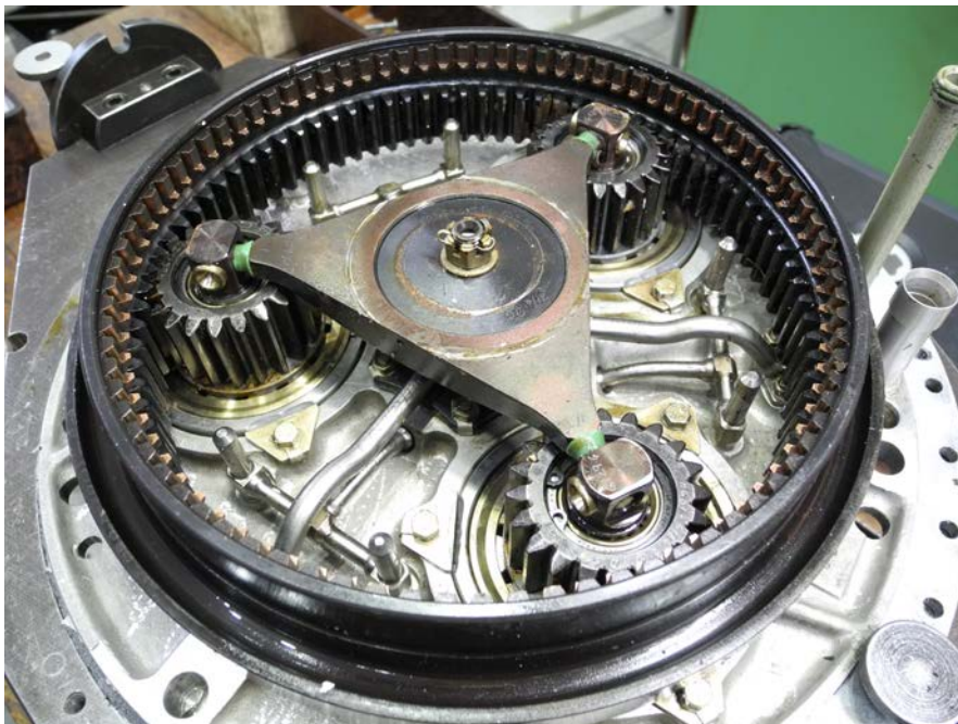
Figure 12 – Ring Gear - Installed
