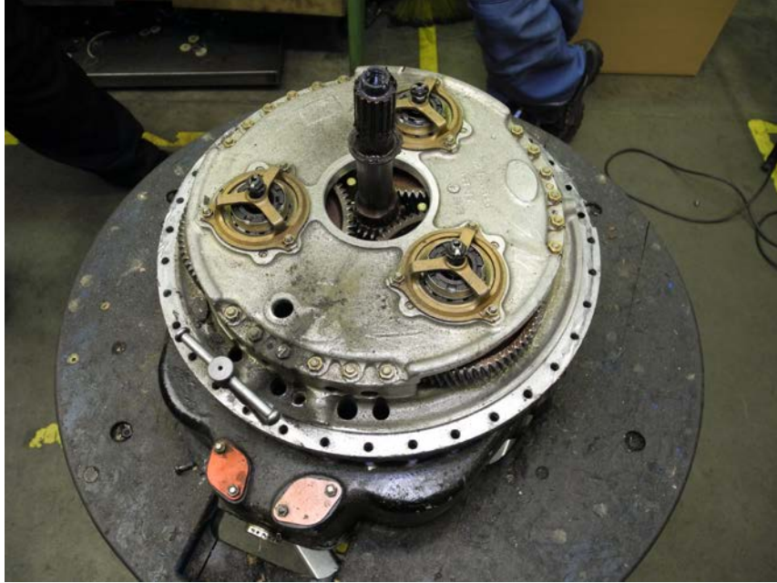
Figure 8 – Quill Shaft - Bent
