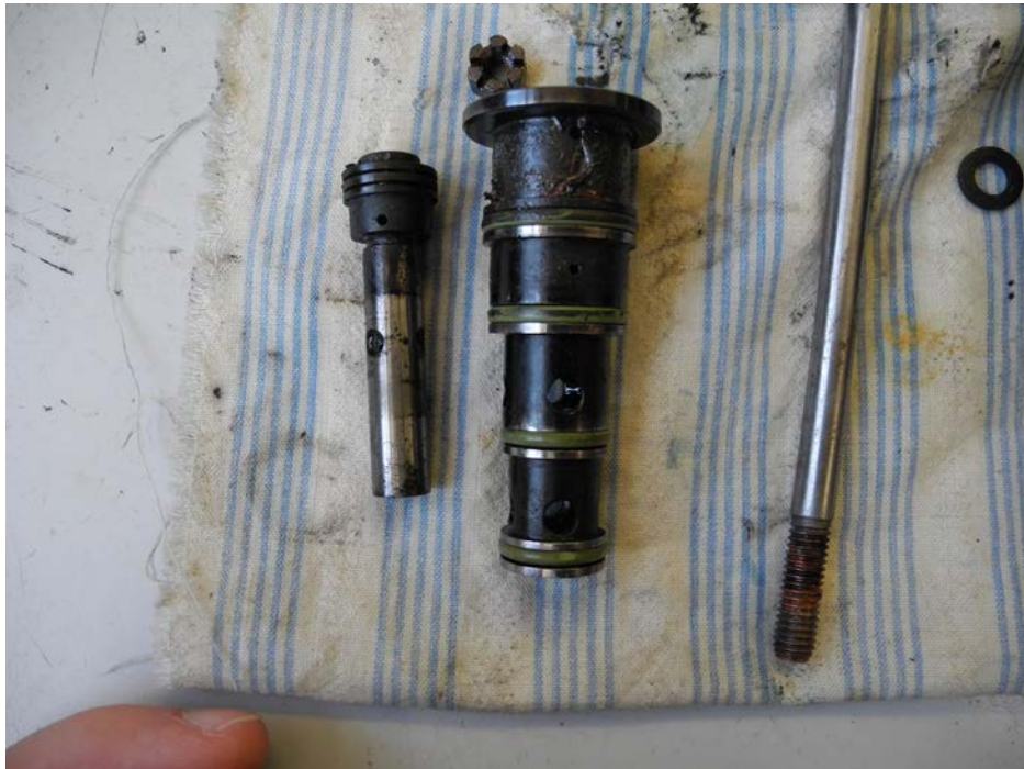
Figure 30 - Emergency Circuit Actuator Valve
