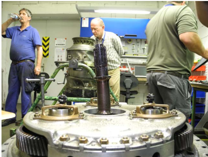
Figure 8 – Quill Shaft - Bent
