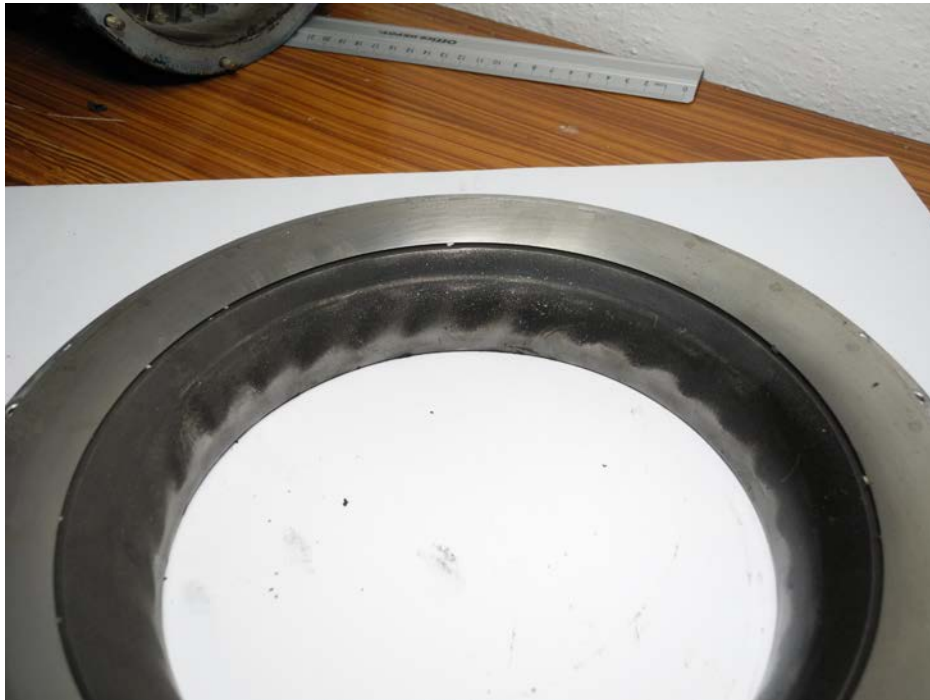
Figure 24 - Impeller Shroud - Rotationally Scored
