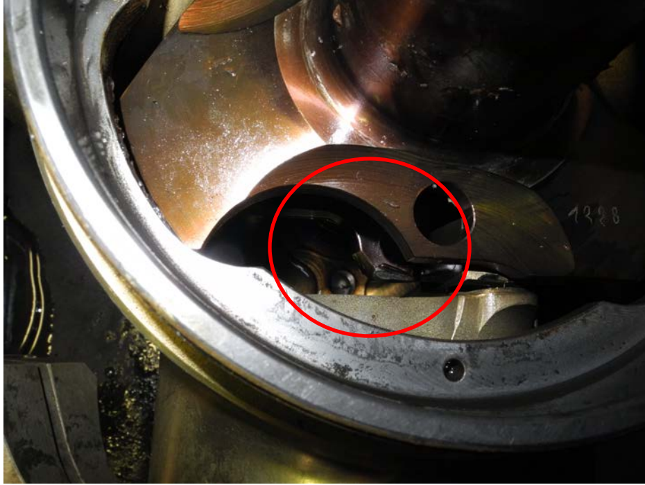
Figure 37 – No. 1 Blade Pitch Actuation Flange On The Piston Fork
