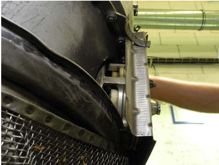
Figure 16 – Bleed Valve – Partially Open
