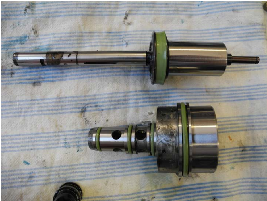
Figure 28 – Main Metering Valve
