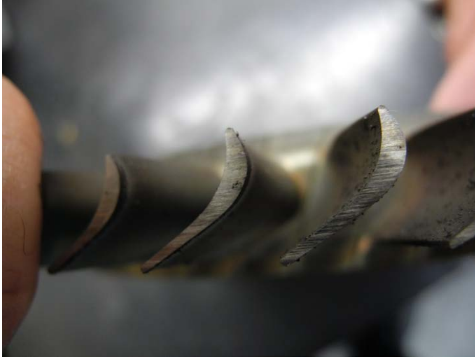
Figure 17 – Gas Generator Turbine Blade Tips – Rotationally Scored
