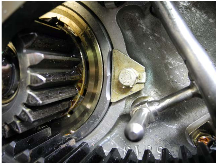
Figure 11 – Spalled Bearing Outer Races
