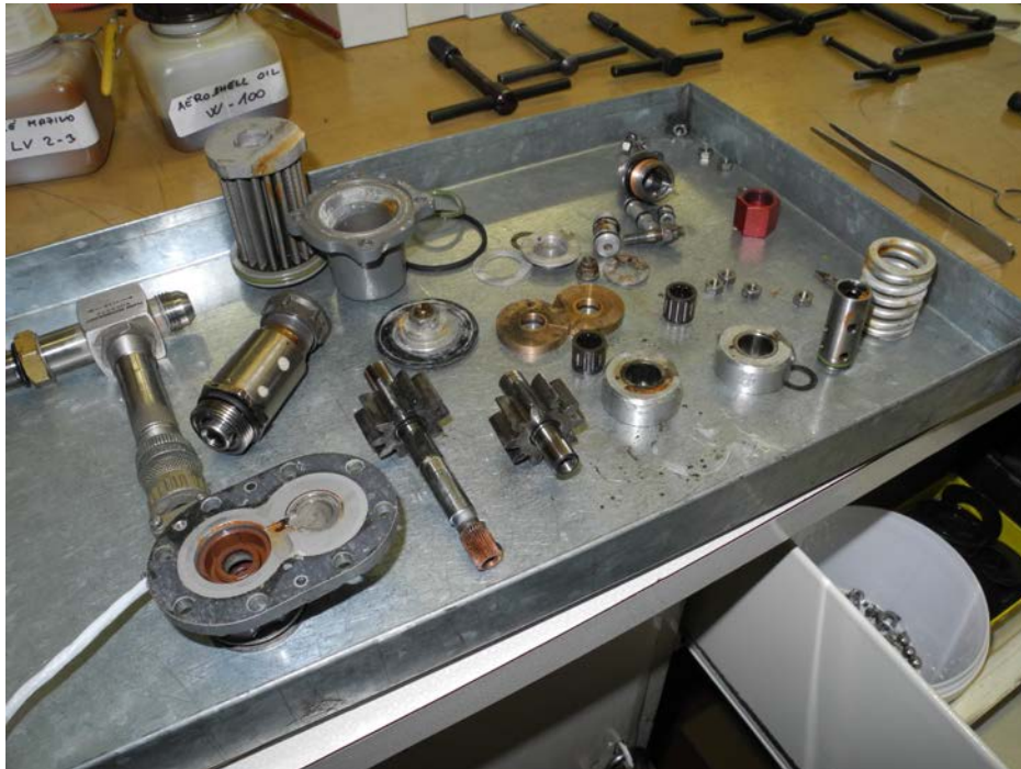
Figure 36 – Complete Fuel Pump Components
