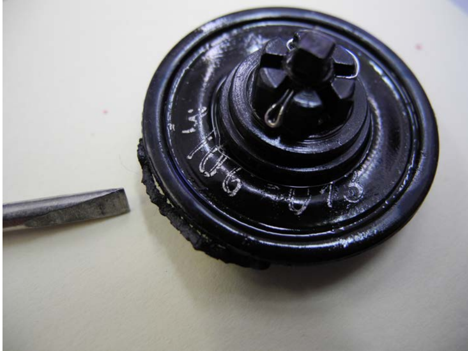
Figure 33 – Flapper Nozzle Rubber/Fabric Diaphragm
