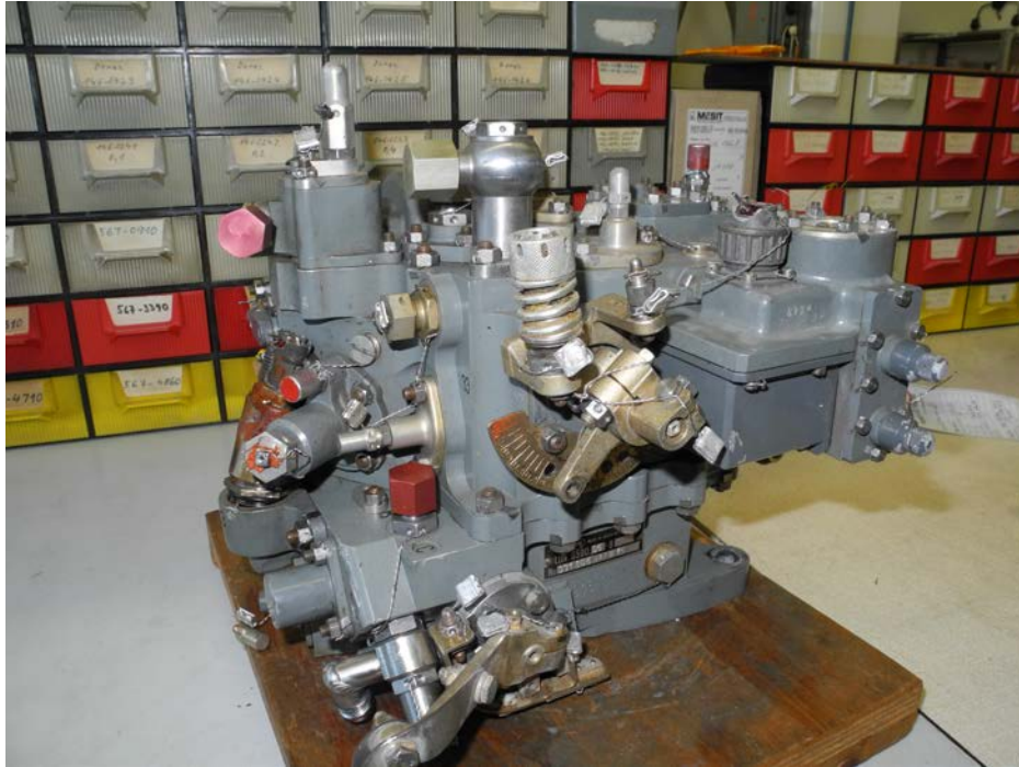
Figure 25 – FCU Prior to Teardown
