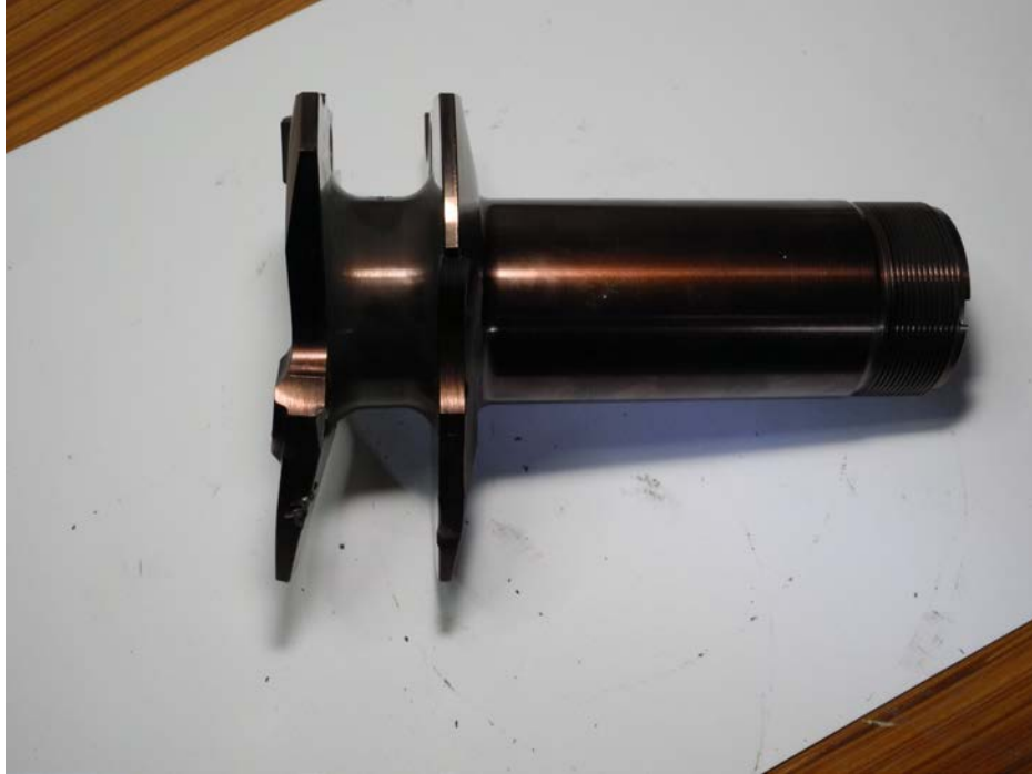
Figure 39 - No. 1 Blade Pitch Actuation Flange On The Piston Fork
