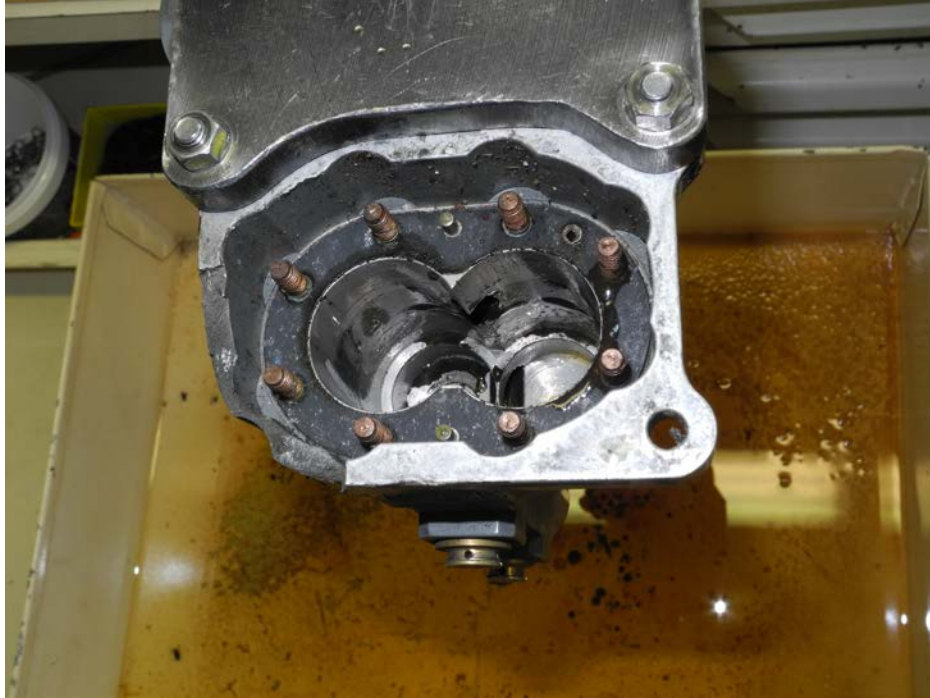
Figure 35 – Fuel Pump Gear Cavity
