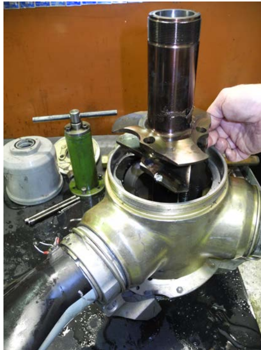
Figure 38 - No. 1 Blade Pitch Actuation Flange On The Piston Fork
