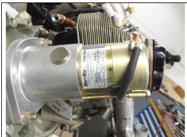
Photo 17: Starter Motor as Viewed on Engine
