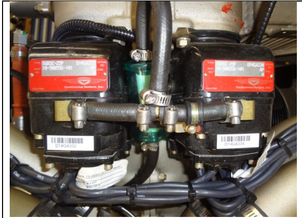
Photo 21: Both Magnetos as Viewed Mounted to Engine
