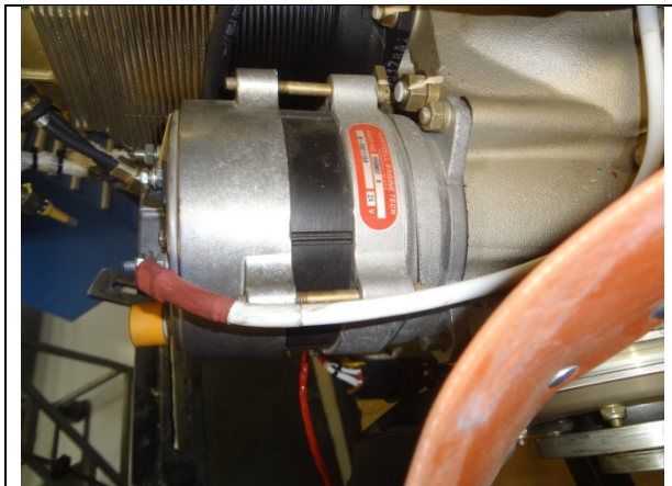
Photo 18: Alternator as Viewed Mounted on Engine
