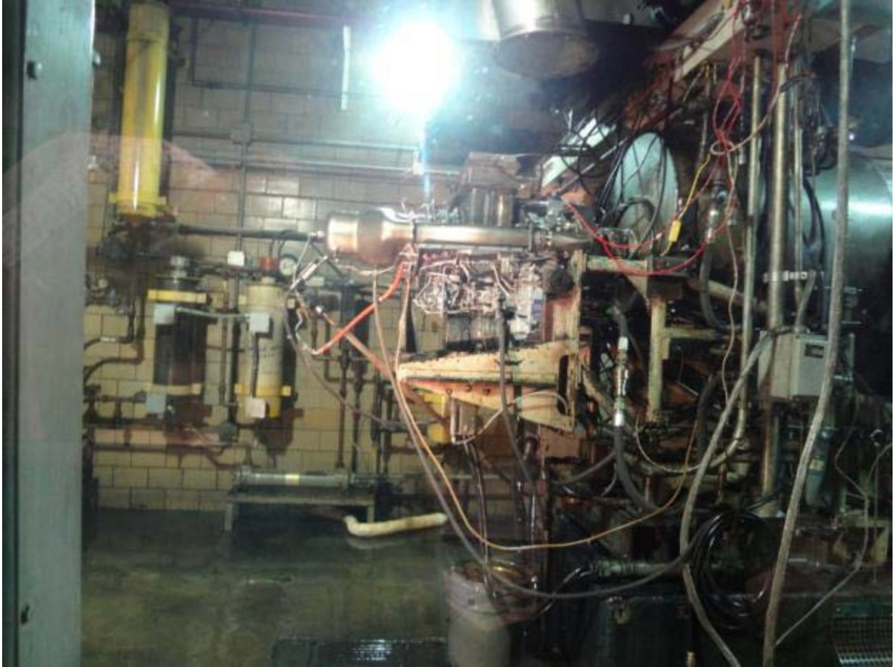
Photo 9: Engine Mounted in Test Stand
