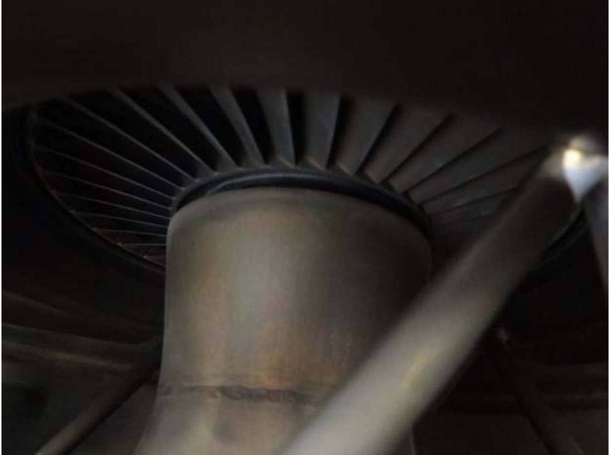
Photo 7: Fourth Stage Turbine Blades as Viewed in Engine on Engine Stand
