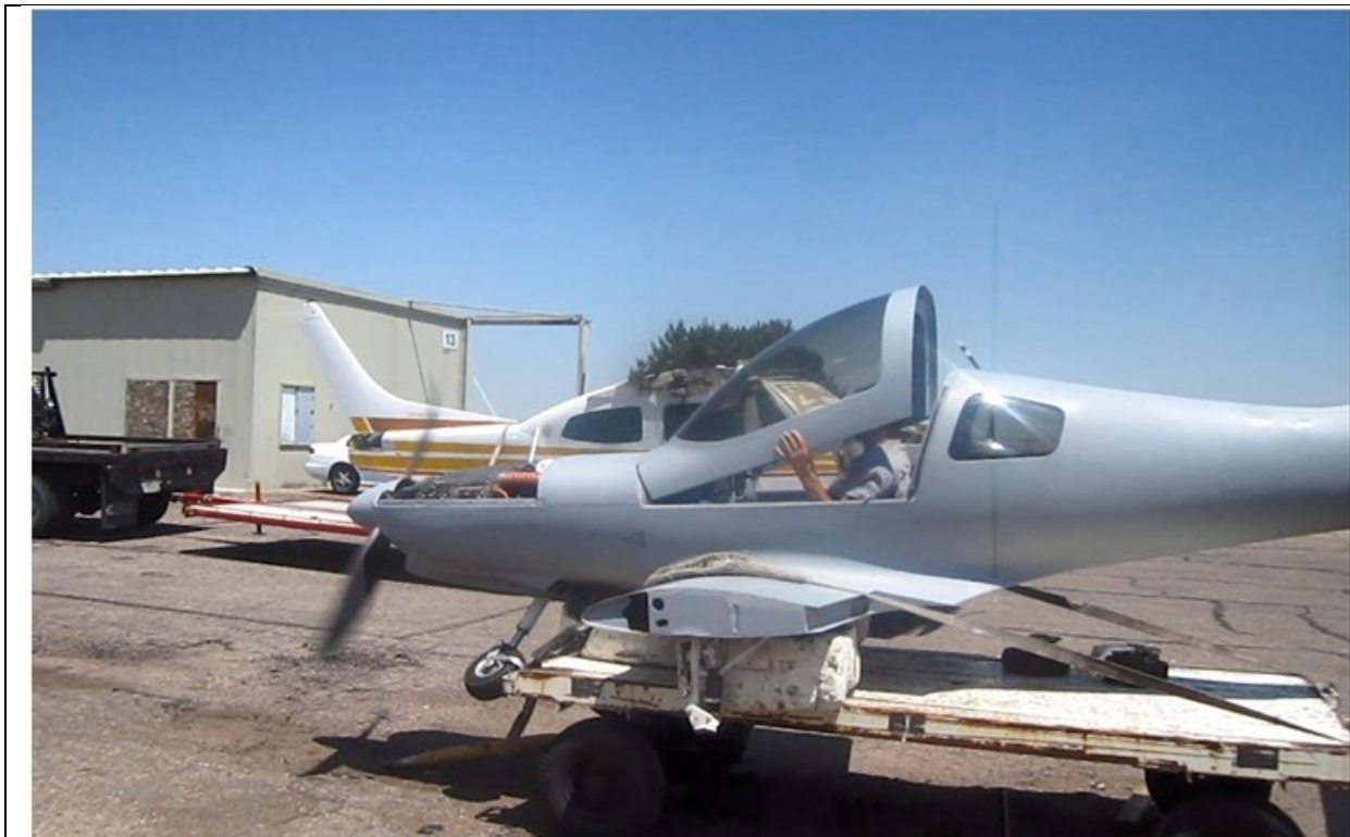
Fuel was added to the airplane header tank. The engine was started and run at various power settings. The magneto drop was “high” but similar between both left and right magnetos.
