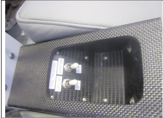
Transfer pumps, for wing fuel tanks
