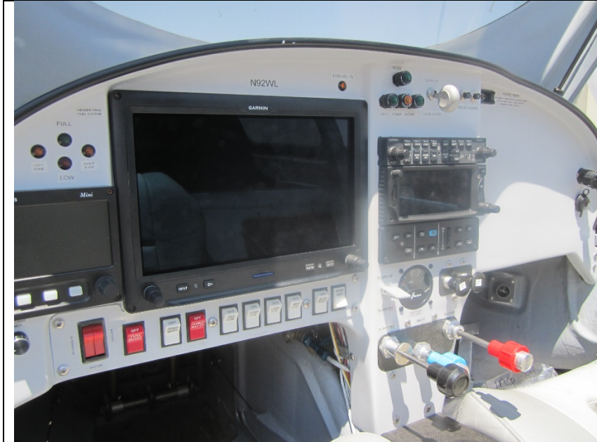
The airplane was equipped with a Garmin EFIS, and “standard” throttle, prop, and mixture controls
