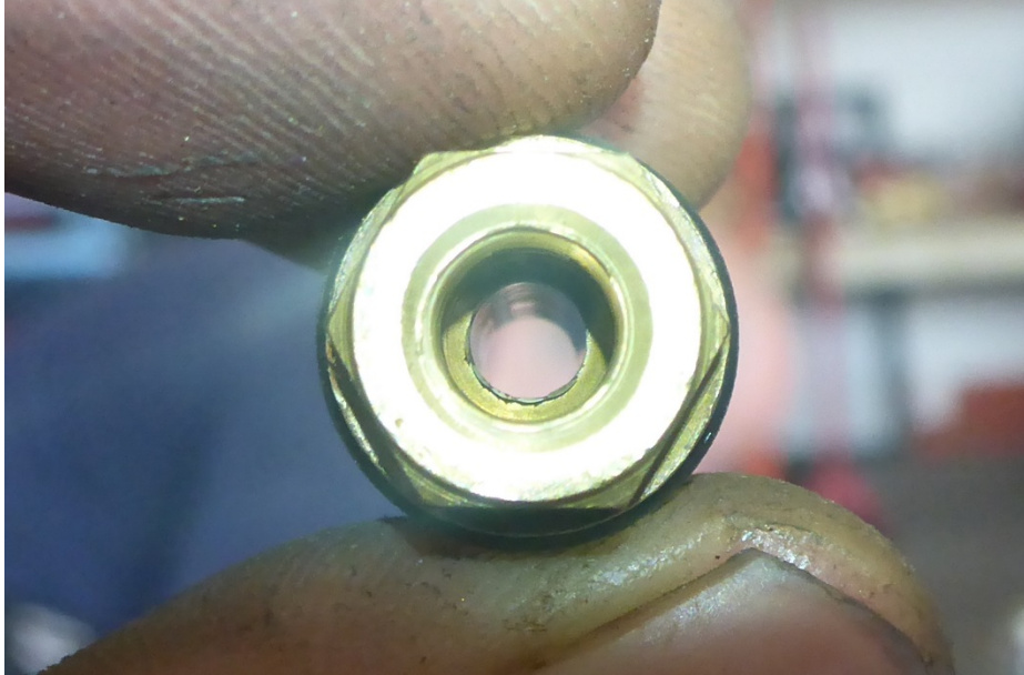
Photo 9 – Left (Cylinders 2/4) Carburetor Mixing Tube Bore
