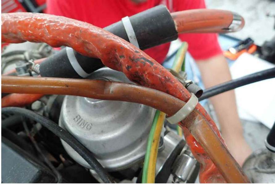
Photo 11 – Coolant Overflow Line
