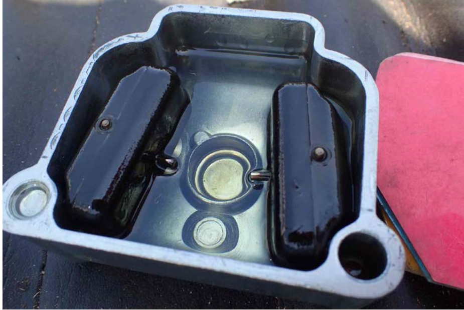
Photo 5 - Left (Cylinders 2/4) Carburetor at Accident Site
