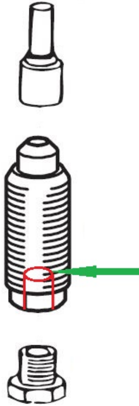
Figure 1 – Left (Cylinders 2/4) Carburetor Mixing Tube Bore Showing Burr Location
