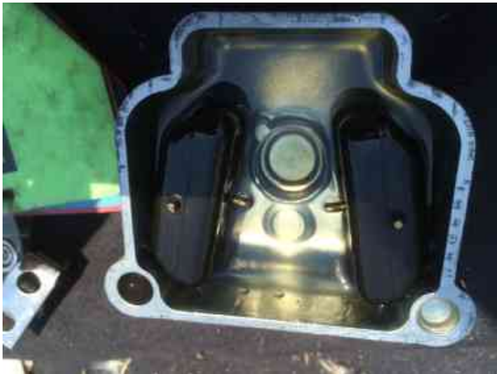
Photo 4 – Right (Cylinders 1/3) Carburetor at Accident Site
