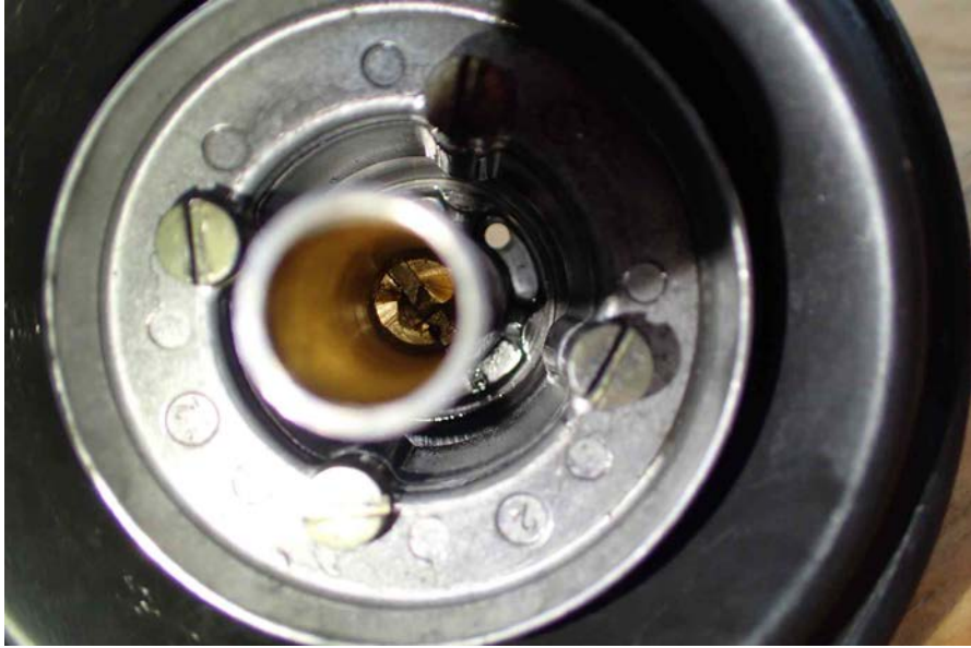
Photo 17 –Left (Cylinders 2/4) Carburetor Fixation Screw Head
