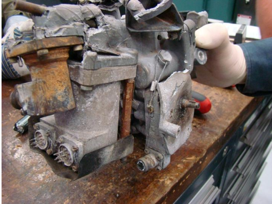
Figure 10 - Fuel metering unit (HMU)
