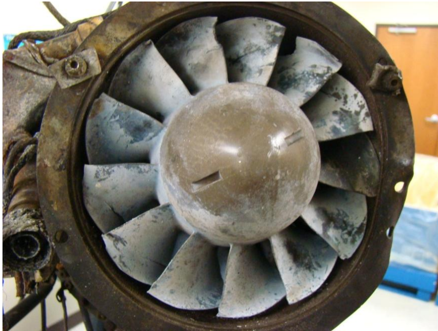
Figure 4 - Module M02 – Axial compressor
