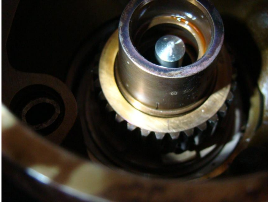
Figure 9 - Splined nut pinion coupling, 2 mm displacement
