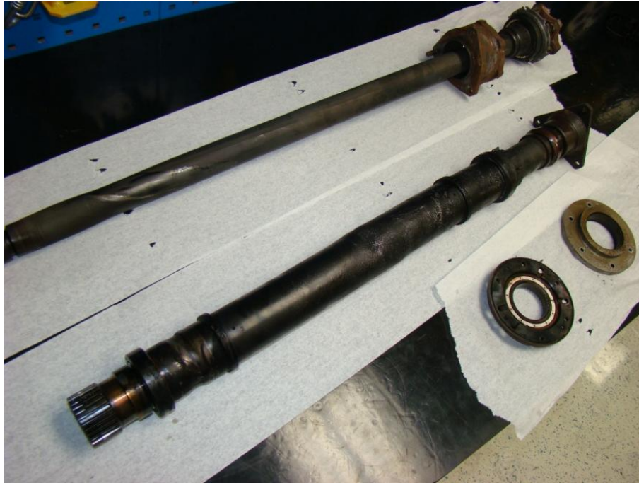
Figure 3 - The freewheel shaft (top) and power transmission shaft (bottom)
