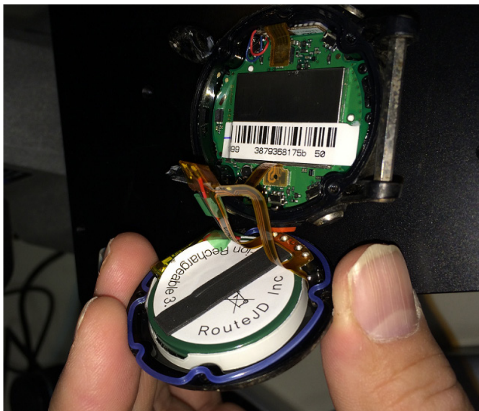
Figure 2. Garmin D2 watch, internal inspection.
