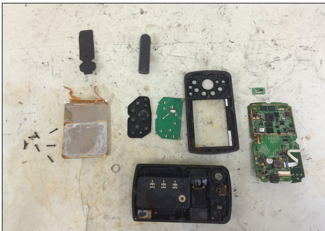
Figure 7. Garmin GPSMAP 396 disassembled.
