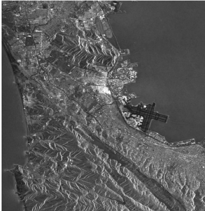
Figure 18. Multi-image reflectivity map of the ERS descending dataset extending over the San Bruno area.
