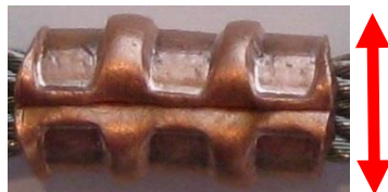
Post Accident Test 5/32 Cable, 18-4-P Sleeve, compressed with 5/32 Swage Tool
