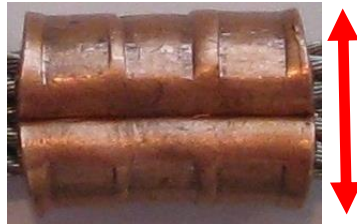
Post Accident Test 5/32 Cable, 18-4-P Sleeve, compressed with 3/16 Swage Tool
