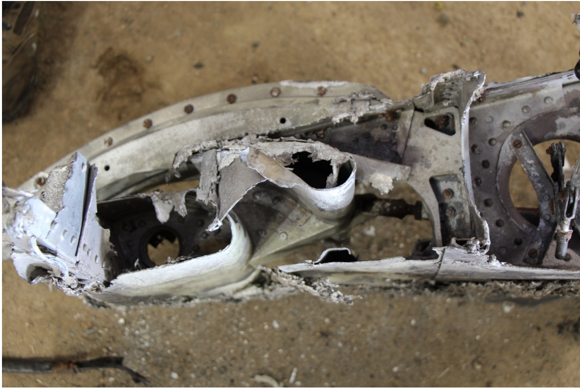
Photograph 6: Right wing flap track
