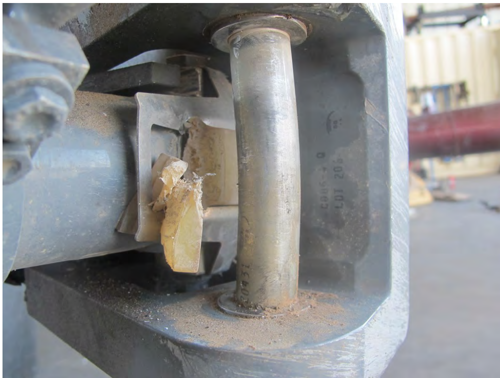
Photo 9 Teeter Stop and Coning Bolt of Separated Blade
