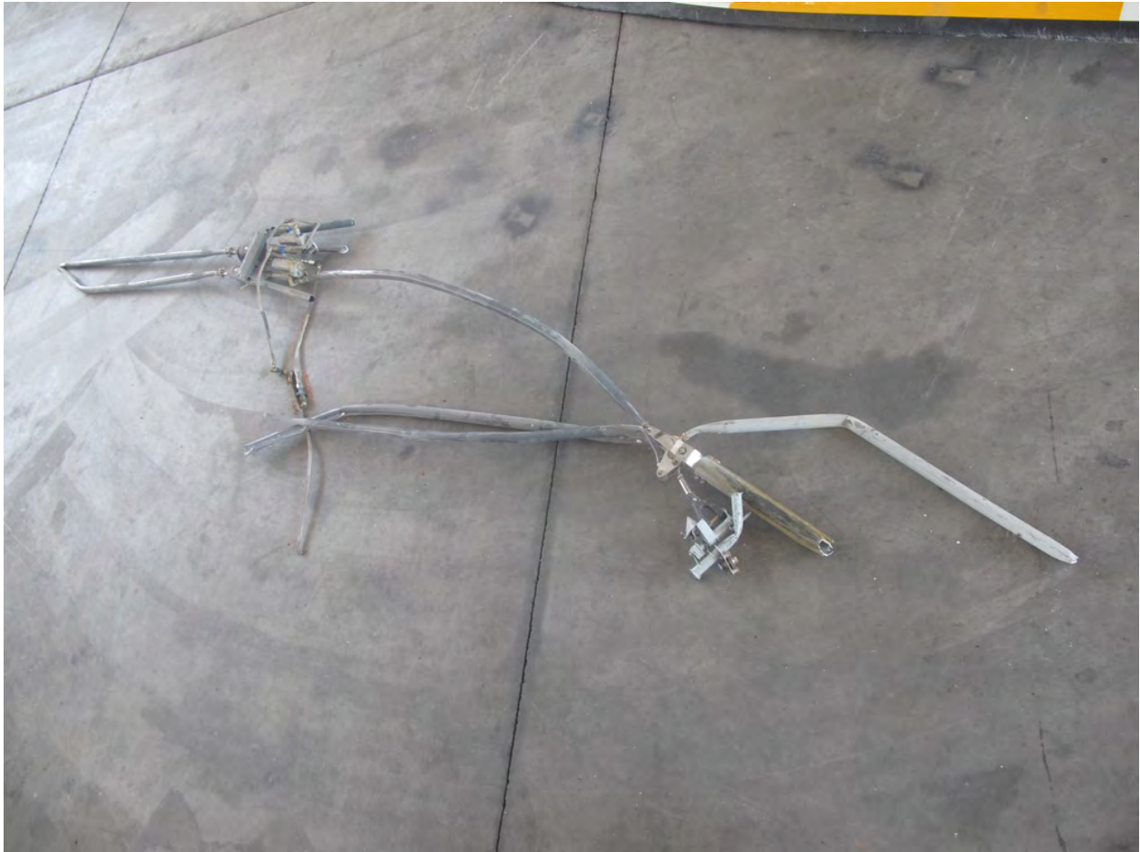
Photo 1 Main Rotor Flight Controls
