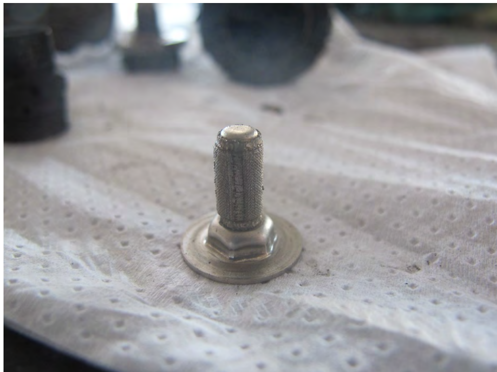
Photo 20 Fuel Spray Nozzle Filter
