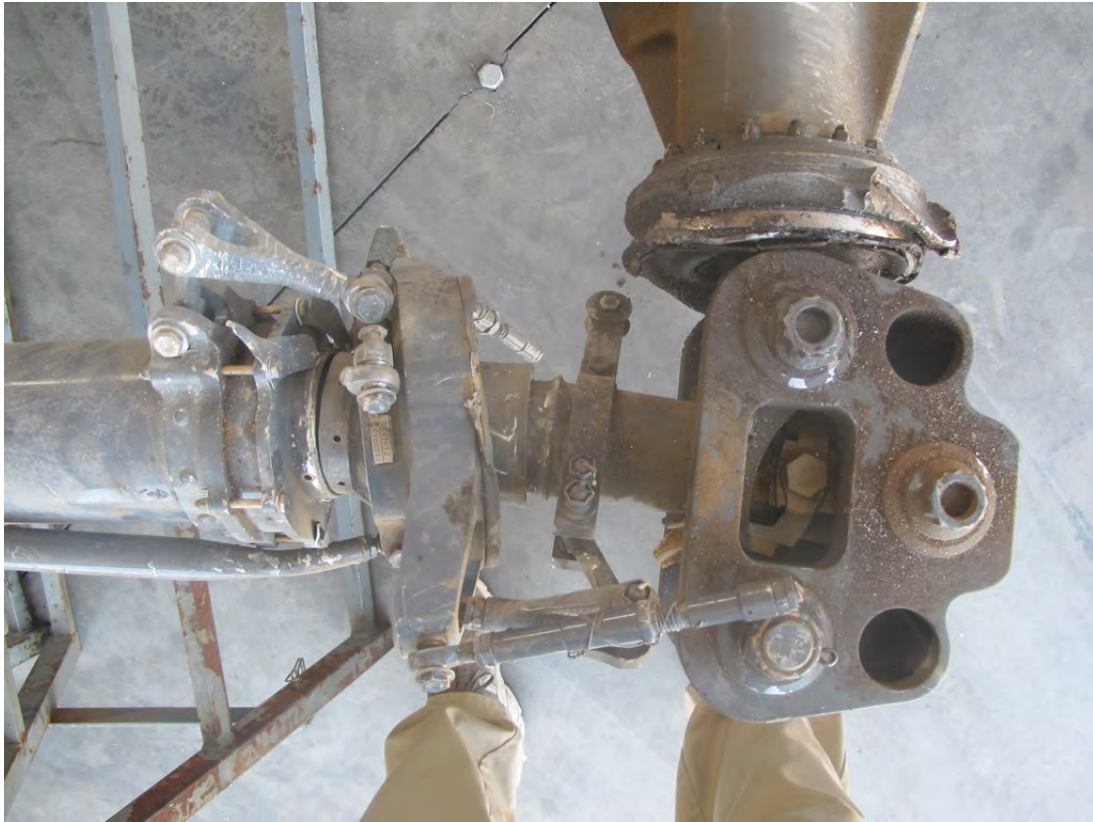
Photo 10 Bent Main Rotor Drive Shaft
