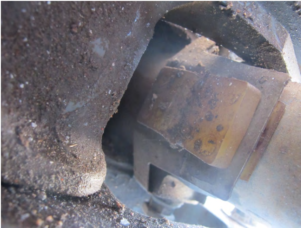
Photo 8 Teeter Stop of Attached Blade
