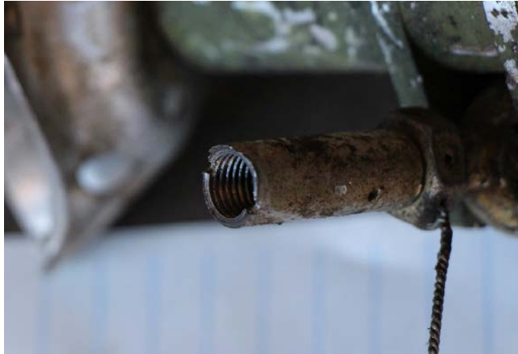
Photograph 4: View of Left Aileron Bell Crank Push/Pull Tube Rod End
