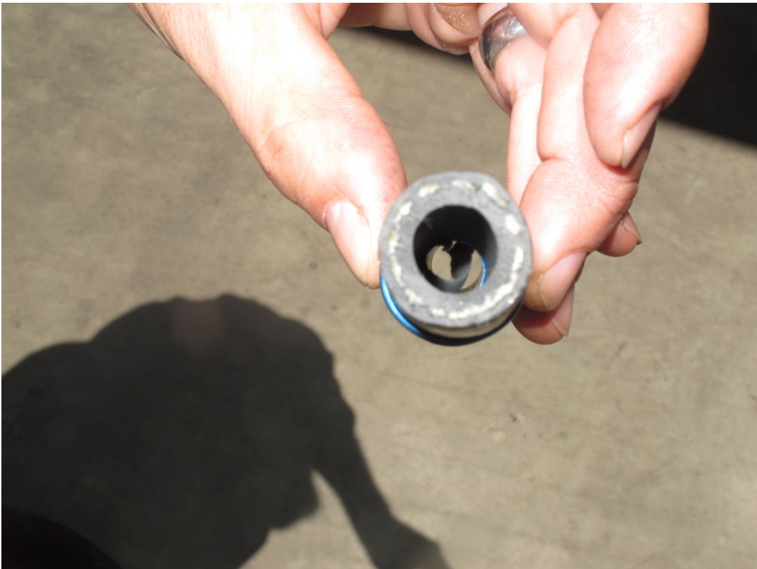
Photo 17 Obstruction in Hose
