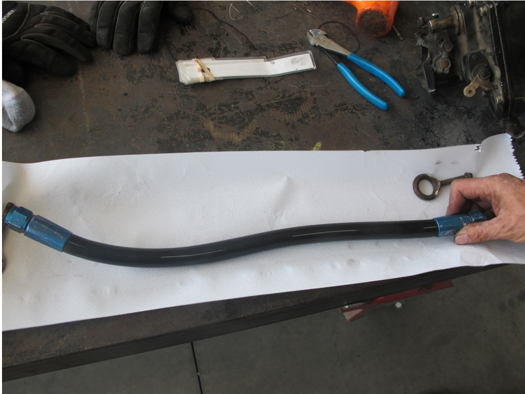
Photo 14 Line from Gascolator to Carburetor with Firesleeve Removed
