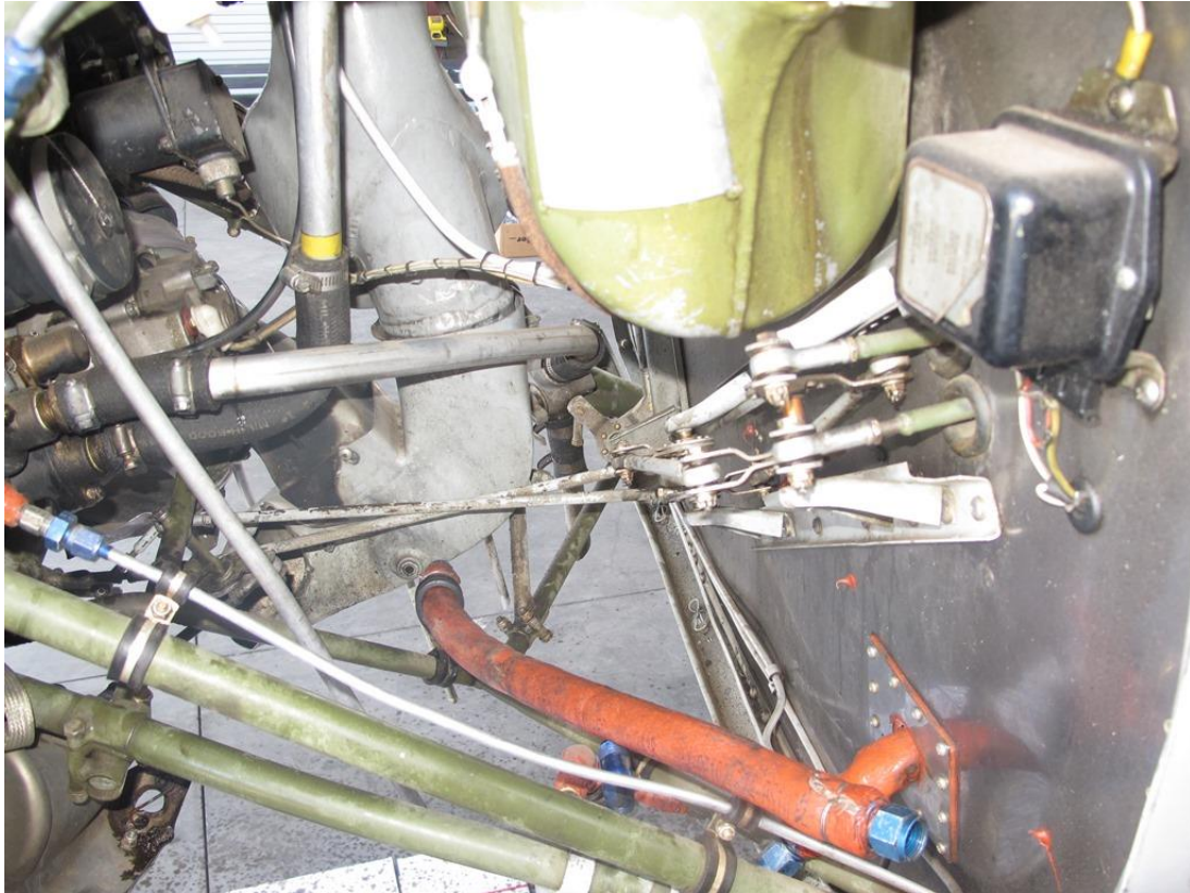
Photo 13 Fuel Line from Gascolator to Carburetor
