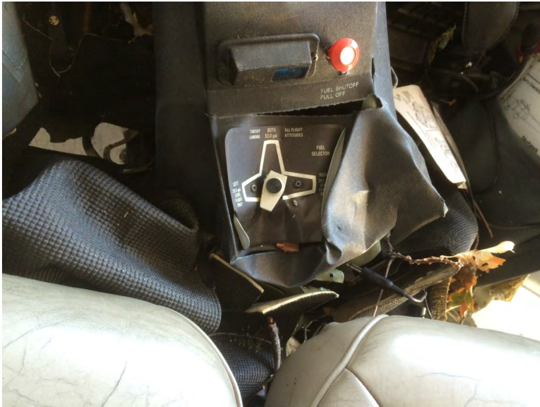
Photo 8 Fuel Selector Valve
