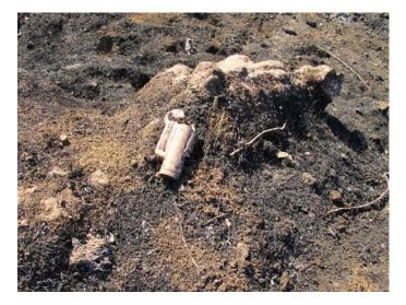
The aft seatbelt buckle assembly was found loose from the lap belt attachment and both shoulder belt attachments. The forward seatbelt buckle assembly including lap belt attachment both shoulder belt attachments were attached and securely buckled. The majority of the seatbelt webbing was consumed by fire.
