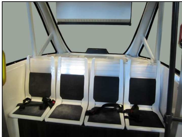
Figure 4. Seats equipped with lap belts, shuttle interior (photo taken 3 days after collision).
