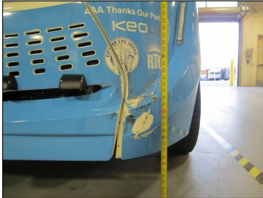
Figure 8. Closeup of damage to lower left front of shuttle (photo taken 3 days after collision).
