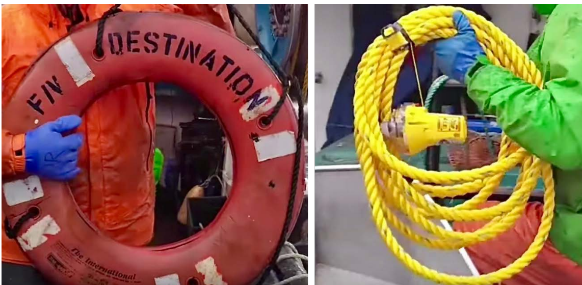
Screenshots from video captured by the Silver Spray crew of items recovered from the Destination : a life ring (at left), along with a line and the vessel’s EPIRB (at right).
