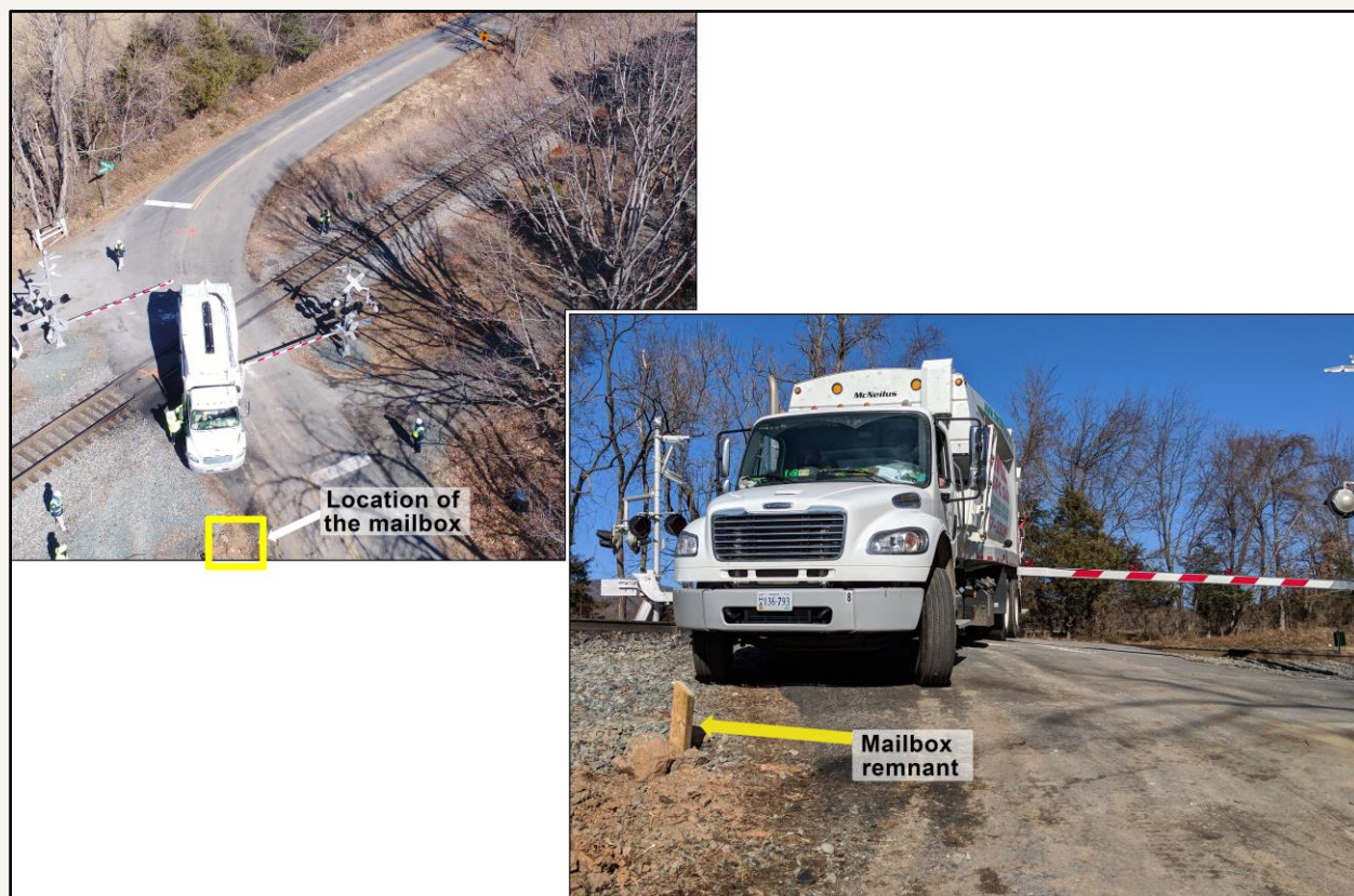
Figure 5. Overhead (top) and front (bottom) views of exemplar truck at position similar to that of crash truck at time of impact; also shown are locations of mailbox and remnant of mailbox post.
