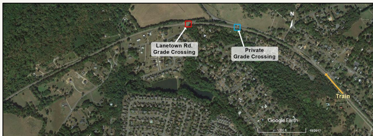
Figure 3. Overhead view of railroad tracks in crash area, showing grade crossings and track geometry. (Source: Adapted from Google Earth)
