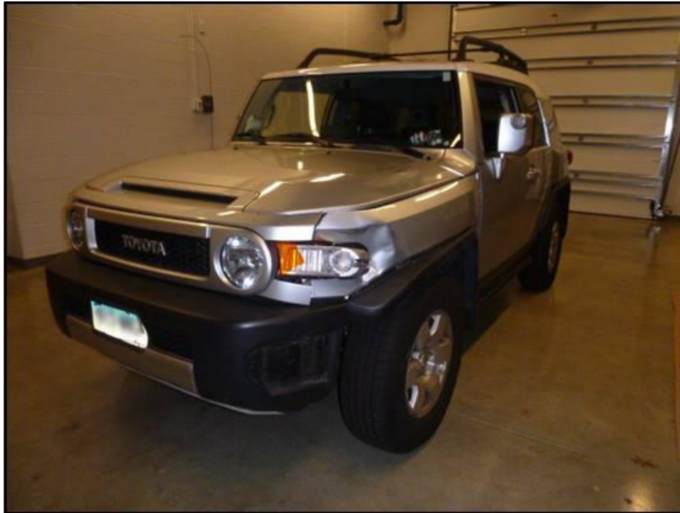
Figure 3. Front view of crash SUV showing damage to left fender near turn signal assembly.
