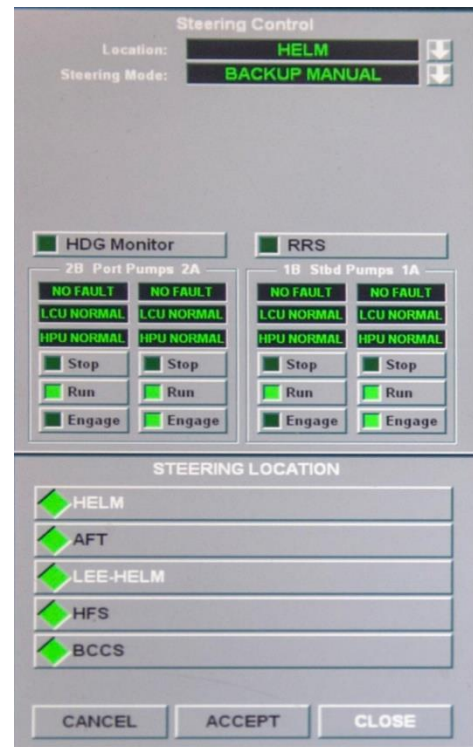
Figure 5. Steering control region of IBNS GUI display, with opened steering location menu. (From US Navy photo)
