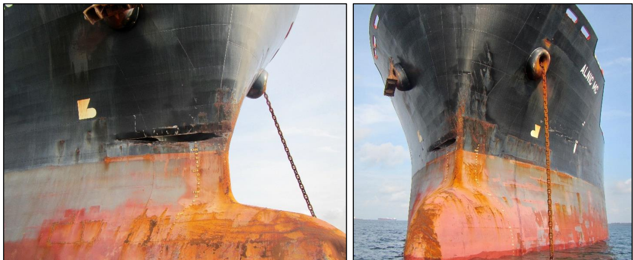
Figure 13. Hull damage to Alnic MC . (Photos by Coast Guard)
