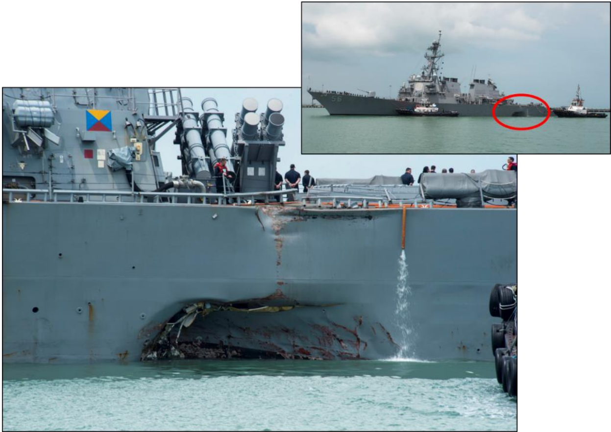
Figure 12. Hull damage to John S McCain . (Photos by Navy Mass Communication Specialist 2nd Class Joshua Fulton)
