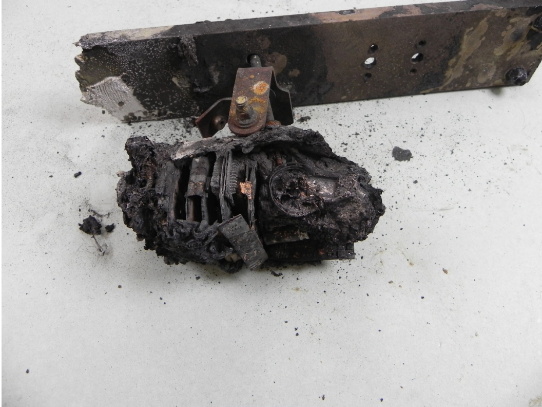
Figure 6a. Postaccident condition of onboard image recorder.
