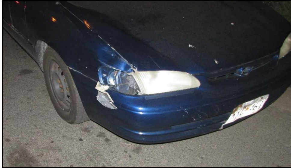
Figure 5. Damage to 1998 Toyota Corolla traveling straight at reported speed of 33 mph, Riverdale Park, Maryland, April 2016 (NTSB 2018a).
