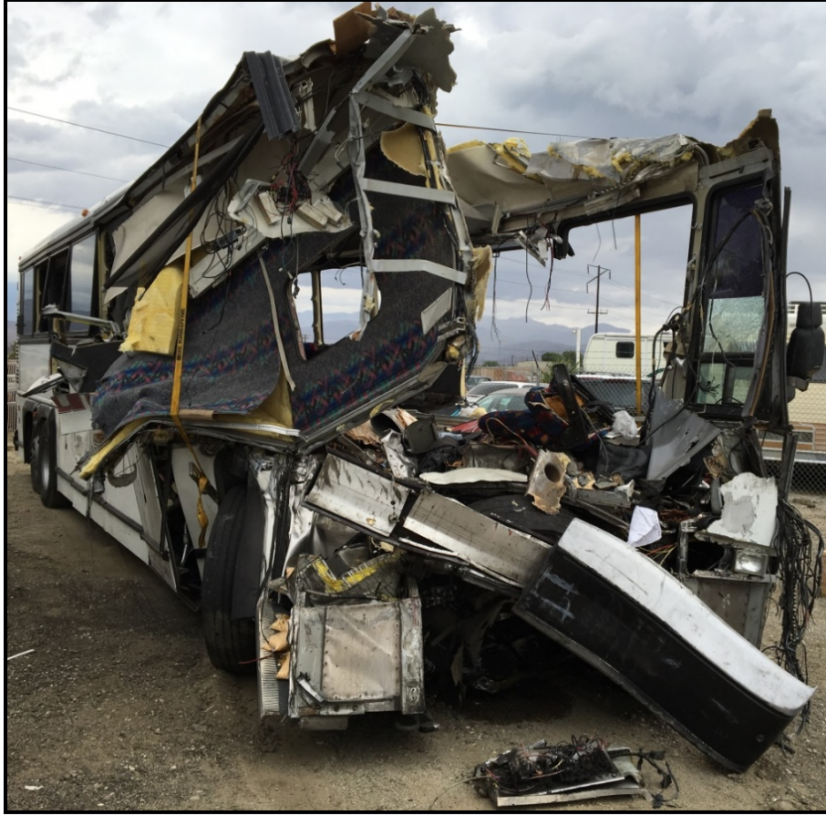
Figure 8. Bus postcrash, showing extensive damage to the front of the vehicle.
