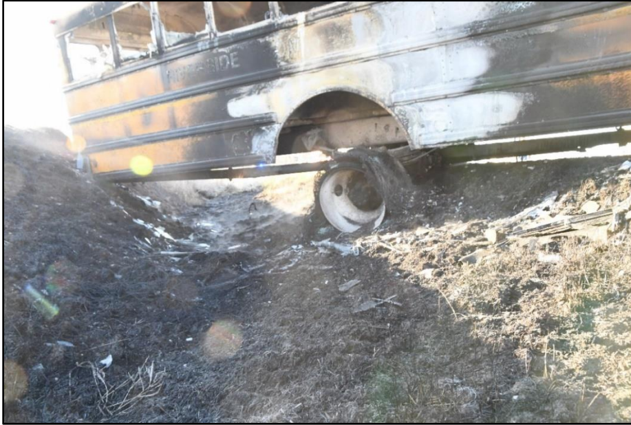
Figure 9. Right rear bumper of bus embedded in drainage ditch embankment.
