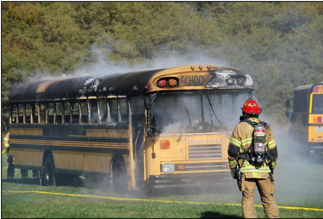
Figure 16. Extent of damage to school bus in Kansas City fire demonstration. (Source: NAPT)
