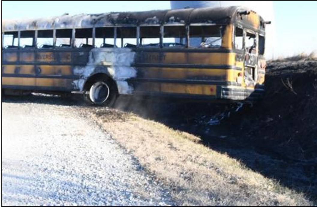
Figure 5. Burned school bus (left rear) at final rest in ditch. (Source: Pottawattamie County Sheriff's Office)
