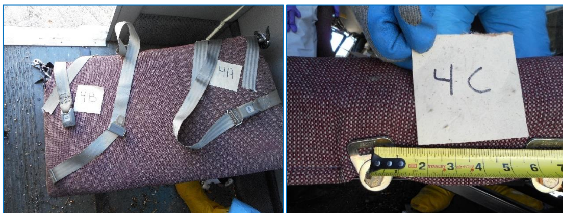
Figure 6. Fourth-row bench seat (left) and closeup view of lap belt anchorage points (right).
