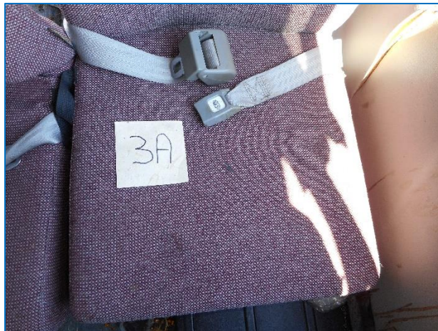
Figure 5. Lap belt assembly in seat 3A, showing traveling retractor with latch and buckle.
