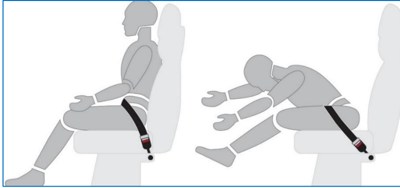
Figure 14. Depiction of motion of lap-belted occupant in frontal collision.
