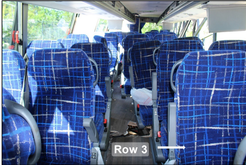
Figure 5. Motorcoach interior, showing the buckling of the floor and the lateral displacement of the seats.
