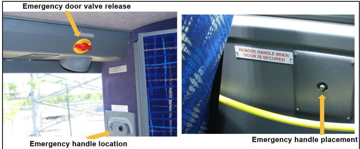
Figure 6. Interior of the motorcoach, showing the three assemblies necessary to open the rear door.
