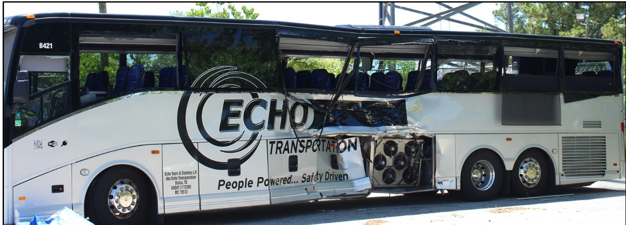
Figure 4. Motorcoach postcrash, showing contact damage to the left side.
