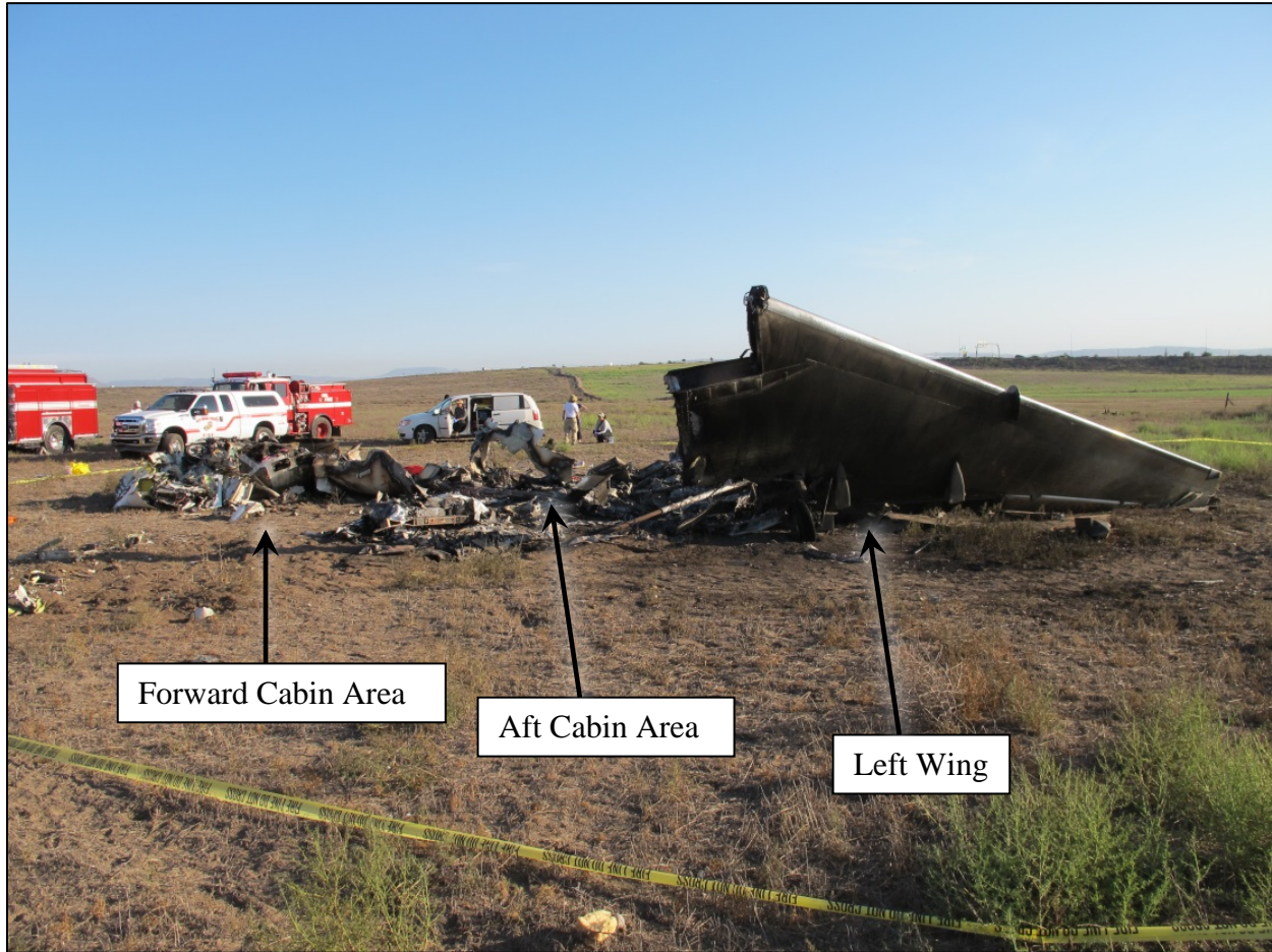
Figure 5-Sabreliner's Main Wreckage (South View)
