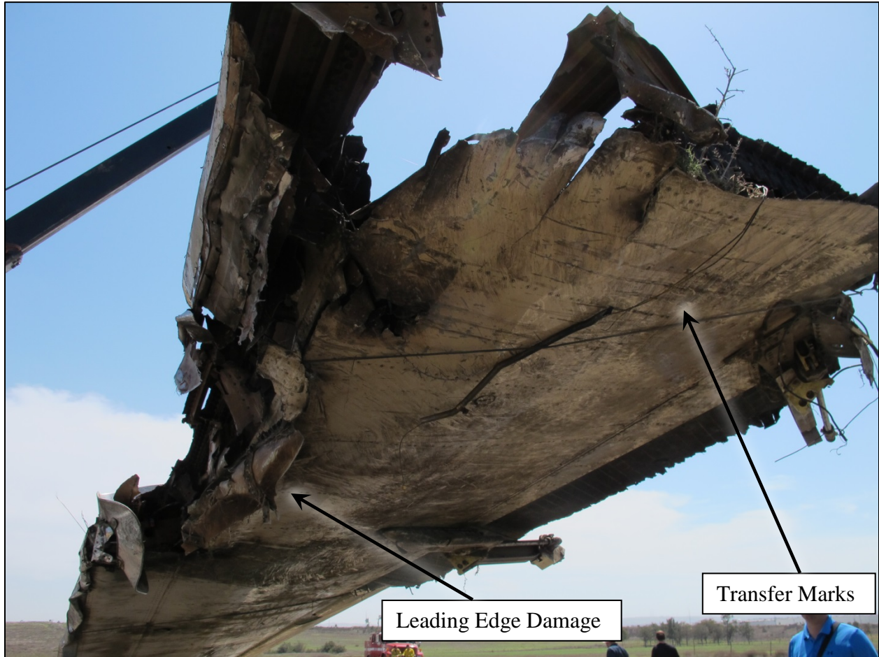
Figure 7-Sabreliner's Right Wing (leading edge damage)
