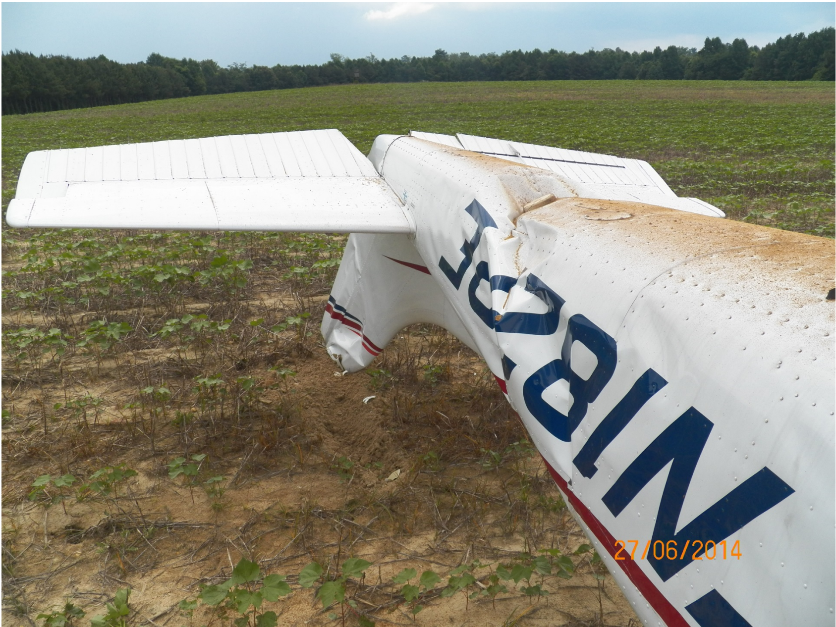
Photo 7 - View of empennage crush damage
