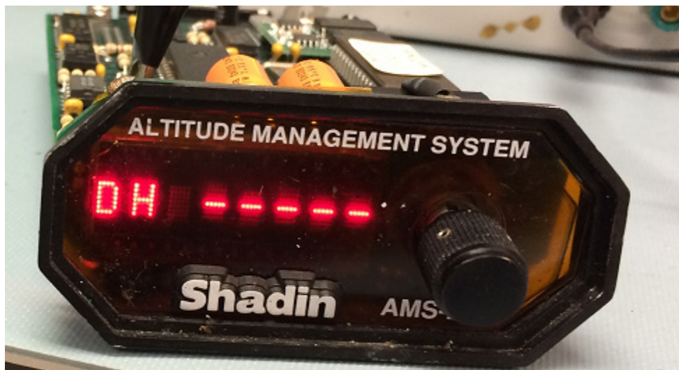
Figure 2. Shadin Altitude Alert System example display of decision height.
