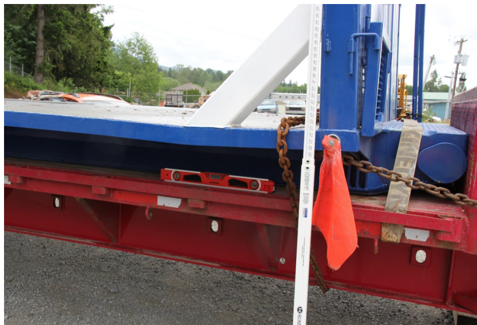
Photograph 9: Digital level positioned to obtain angle of trailer which is a similar angle as the base of the load.
