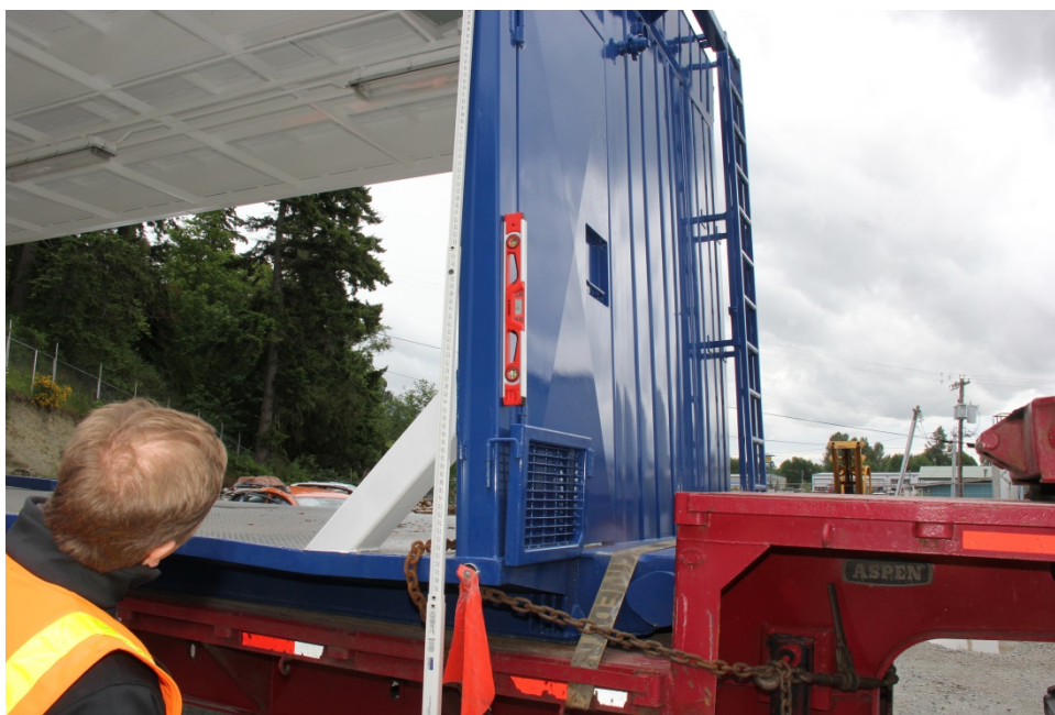
Photograph 11: Digital level positioned to obtain the angle of the front surface of the load.
