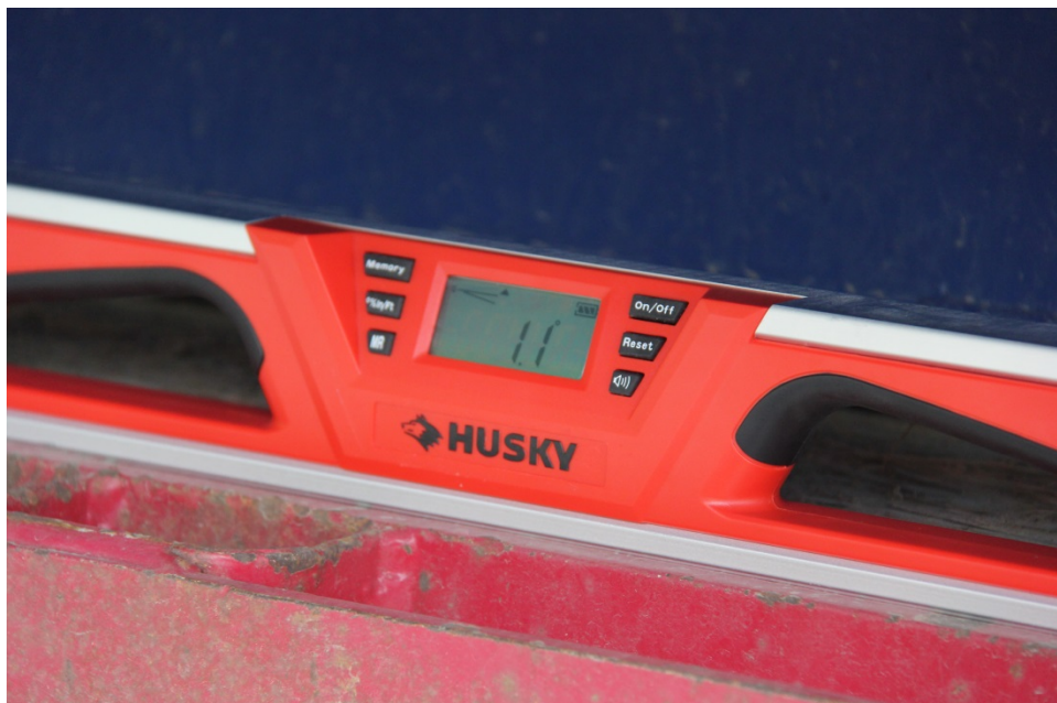
Photograph 10: Trailer is sloping 1.1 degrees downward toward the front of the trailer.
