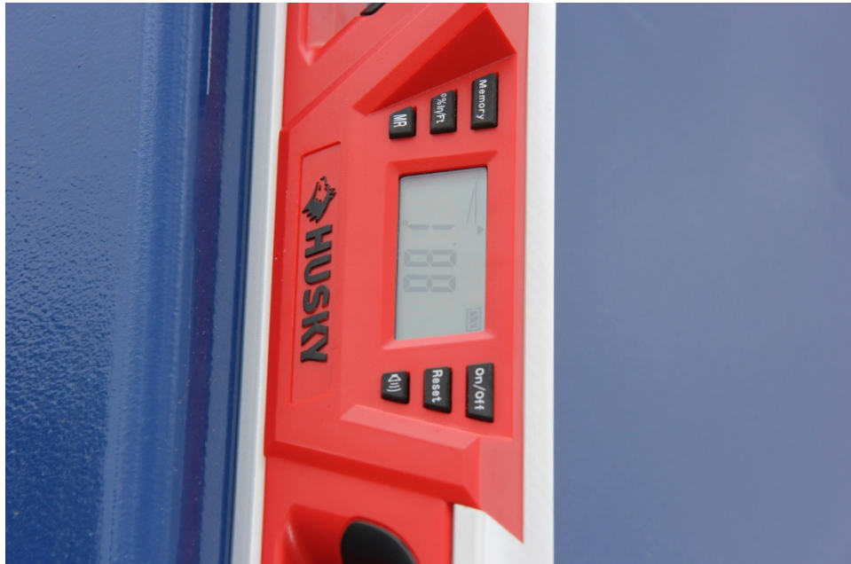
Photograph 12: Angle of the front surface of the load is 88.1 degrees (1.9 degrees from vertical) tilted toward the rear of the trailer. The total approximate angle is 3.0 degrees (1.1 plus 1.9).
